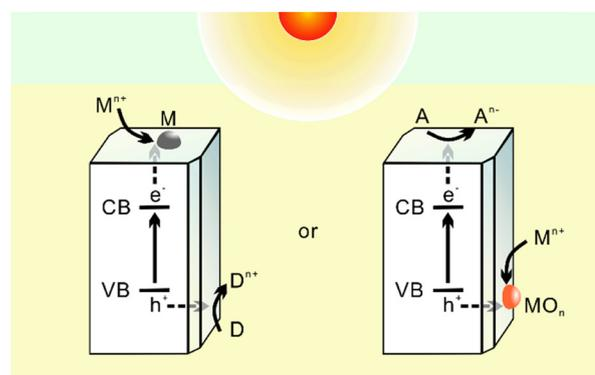
Fig. 1 Schematic diagram of reductive or oxidative photodeposition. VB: valence band, CB: conduction band, M: metal, D: electron donor, A: electron acceptor, and *n*: number of electrons (or holes) involved.
