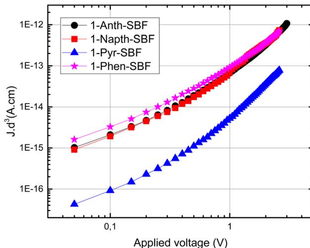
Fig. 9 SCLC device (left): thickness-scaled current–voltage characteristics of **1-Napht-SBF**, **1-Phen-SBF**, **1-Anth-SBF** and **1-Pyr-SBF** hole-only SCLC devices (right): The dotted lines indicate the SCLC regime and the continuous ones indicate the Ohmic regime.
