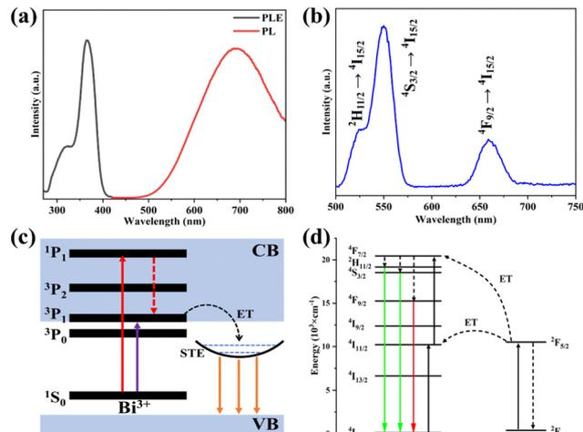
Fig. 3 PL properties of 2%Bi@20%Yb, 7%Er. (a) PL ( $\lambda_{\text{ex}} = 370$  nm) and PLE ( $\lambda_{\text{em}} = 690$  nm) spectra; (b) PL ( $\lambda_{\text{ex}} = 980$  nm) spectrum; (c) schematic diagram of the energy-transfer mechanism of  $\text{Bi}^{3+}$  in core-shell NCs; (d) schematic diagram of the energy-transfer mechanism of  $\text{Yb}^{3+}$ - $\text{Er}^{3+}$  in core-shell NCs.
