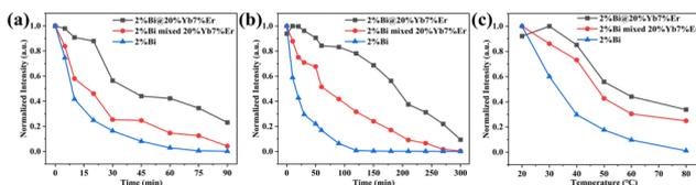
**Fig. 5** Comparison of the PL intensity of 2%Bi@20%Yb, 7%Er core-shell NCs, the mixture of 2%Bi NCs and 20%Yb, 7%Er NCs and 2%Bi NCs under 370 nm excitation: (a) in cyclohexane and DI water ( $v/v = 1:9$ ) mixed solvents under 370 nm excitation; (b) under continuous UV light irradiation; (c) at different temperatures.
