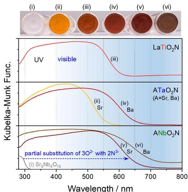
Fig. 2 Photographic images and UV-vis diffuse reflectance spectroscopy (DRS) spectra of perovskite oxynitrides  $\text{AB}(\text{O},\text{N})_3$  ( $\text{A} = \text{Sr}, \text{Ba}, \text{ or } \text{La}$  and  $\text{B} = \text{Ti}, \text{Ta}, \text{ or } \text{Nb}$ ) prepared via nitridation of layered perovskites  $\text{A}_5\text{B}_4\text{O}_{15}$ .
