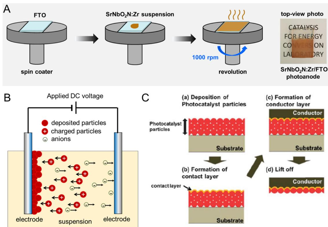
Fig. 11 Particulate photoelectrodes. Schematic diagrams of the preparation of perovskite oxynitride photoanodes *via* (A) spin coating, (B) electrophoretic deposition (EPD), and (C) particle transfer methods. Reproduced with permission.<sup>104</sup> Copyright 2013, RSC. Reproduced with permission.<sup>105</sup> Copyright 2023, Elsevier.
