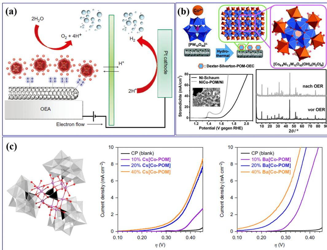
Fig. 3 (a) Scheme for a water-splitting electrocatalytic cell with the integrated nanostructured oxygen-evolving anode of POM/MWCNT.<sup>86</sup> Copyright 2010, Macmillan Publishers. (b) Deposition of Dexter-Silverton polyoxometalate microcrystals on nickel foam electrodes with their OER activity.<sup>87</sup> Copyright 2017, Wiley-VCH. (c) Molecular structure of the Co-POM cluster and electrochemical behavior of Co-POM/CP electrodes.<sup>88</sup> Copyright 2017, Springer Nature.
