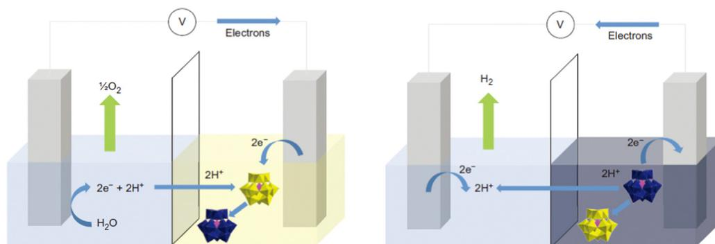
Fig. 1 Schematic of the ECPB-based approach to water splitting.<sup>71</sup> Copyright 2013, Springer Nature.
