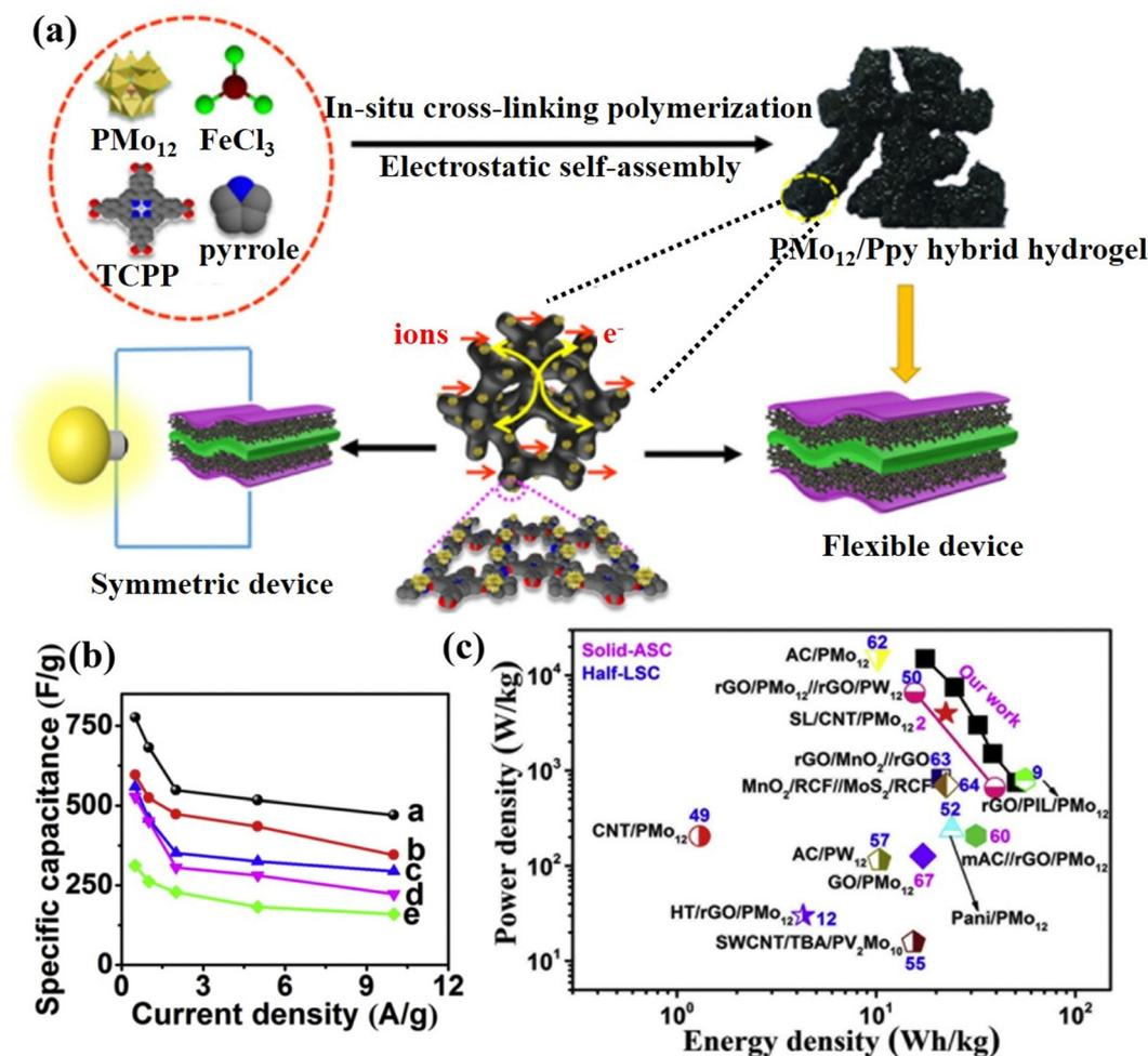
Fig. 22 (a) The preparation process for the PMo<sub>12</sub>/PPy hybrid hydrogel for SCs. (b) Specific capacitances of the prepared samples at various current densities. (c) Ragone plots of the P<sub>2</sub>-PPy gel//P<sub>2</sub>-PPy gel device compared with the values reported for other devices.<sup>203</sup> Copyright 2019, Elsevier Ltd.
