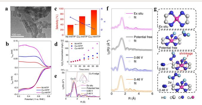
Fig. 3 (a) TEM image of Cu-HHTP. (b) LSV curves. (c) H<sub>2</sub>O<sub>2</sub> selectivity and the electron transfer number of Ni-HITP, Cu-HITP and Cu-HHTP. (d) Cumulative H<sub>2</sub>O<sub>2</sub> yield. (e) FT-XAFS curves for Cu-HHTP. (f) The FT-XAFS fitting results of Cu-HHTP. (g) Scheme of the proposed 2e ORR mechanism for Cu-HHTP. Copyright 2022, Elsevier
