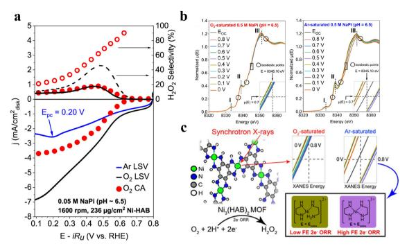
Fig. 4 (a) LSV curves of Ni-HAB. (b) XANES spectra of Ni-HAB/CFP at various applied potentials in O2 saturated and Ar saturated electrolytes. (c) Schematic illustrating the changes in the nickel oxidation state during the 2e-ORR process. Copyright 2022, American Chemical Society.
