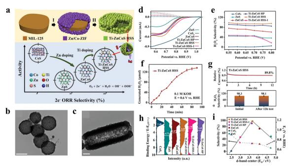
Fig. 10 (a) Illustration of the two-step synthesis of Ti-ZnCoS HSS and the 2e-ORR activity-selectivity of CoSx, ZnS, ZnCoS, and Ti-ZnCoS HSS. (b) and (c) TEM images of Ti-ZnCoS HSS. (d) LSV curves. (e) H<sub>2</sub>O<sub>2</sub> selectivity of all samples in 0.1 M KOH. (f) Valence band spectra. (g) Relationship between selectivity/activity and d-band center. (h) Free-energy diagram for the ORR to  $H_2O_2$ . (i) Scheme presenting the 2e-ORR process over Ti–ZnCoS HSS. Copyright 2022, WILEY-VCH.
