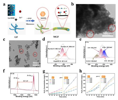
Fig. 8 (a) Schematic showing the synthesis process of MGF. TEM images of (b) MGF and (c) MZIF8. High-resolution XPS spectra of (d) N 1s, (e) O 1s and (f) Zn 2p for MGF. (g)  $H_2O_2$  concentration over the reaction time at various solutions of MGF and GF: (g) pH = 7 (0.5 M  $Na_2SO_4$ ), and (h) pH = 13 (0.1 M KOH). Copyright 2023, American Chemical Society
