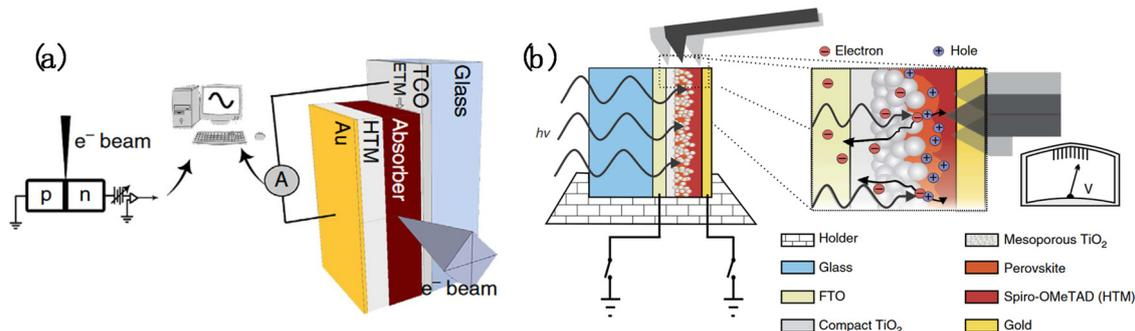
Fig. 3 (a) Illustration of an EBIC experiment on a cross-section of a thin-film solar cell. The electron beam generates e-h pairs in the absorber material, which, after separation, creates a current generation profile inside the cell. TCO, transparent conducting oxide; ETM, electron transporting materials.<sup>31</sup> Copyright 2014, Springer Nature. (b) Schematic diagram of the KPFM measurement principle.<sup>42</sup> Copyright 2014, Springer Nature.
