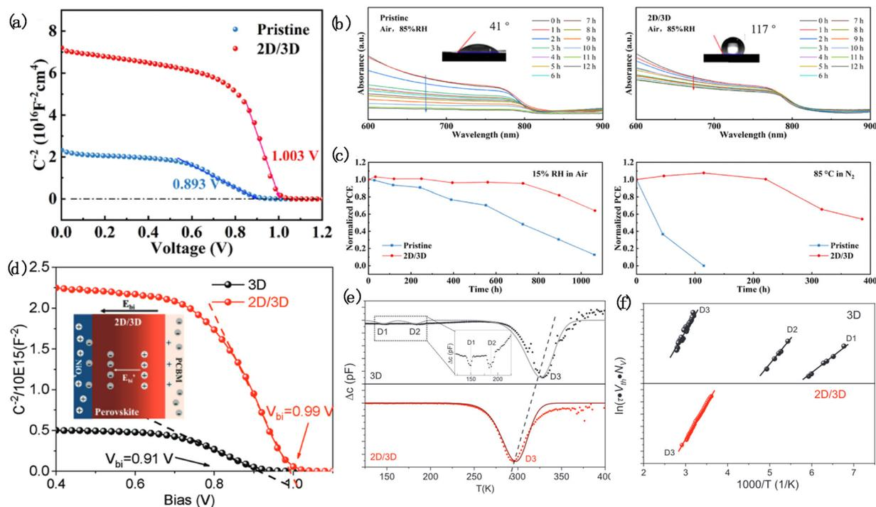
**Fig. 8** (a) Mott–Schottky plots of the pristine and 2D/3D devices. (b) Pristine and 2D/3D perovskite films exposed to ambient air with a relative humidity of 85%. Inset: contact angle images. (c) Normalized PCE of PSCs under wet conditions.<sup>68</sup> Copyright 2022, Elsevier. (d) Schematic illustration of the BEF of the 2D/3D PSCs (inset) and Mott–Schottky curves. (e) DLTS spectra of 3D and 2D/3D PSCs. (f) Arrhenius plots obtained from DLTS signals.<sup>69</sup> Copyright 2022, Wiley.
