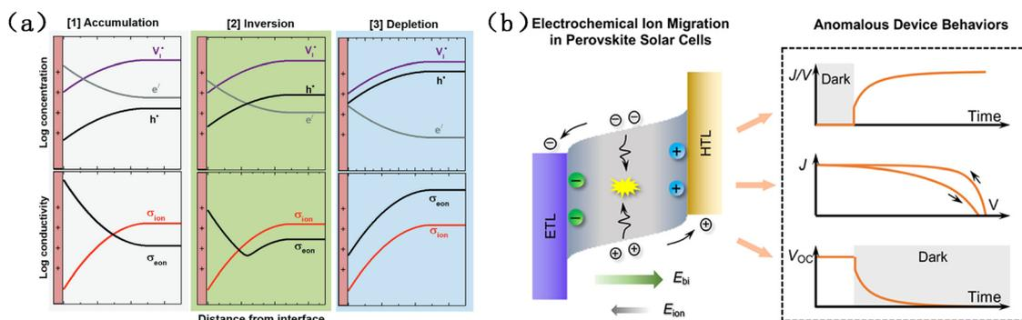
Fig. 20 (a) Schematic concentration and conductivity profiles at the interface.<sup>162</sup> Copyright 2022, Wiley. (b) The anomalous device behaviors caused by electrochemical ion migration.<sup>163</sup> Copyright 2021, ACS.
