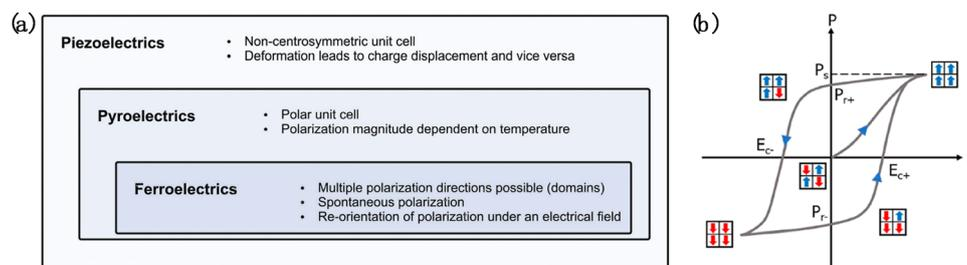
Fig. 17 (a) Diagram of the non-centrosymmetric crystal classes and their ferroic properties.<sup>121</sup> Copyright 2019, Wiley. (b) Schematic illustration of the hysteresis loop for electric displacement versus electric field.<sup>126</sup> Copyright 2023, ACS.
