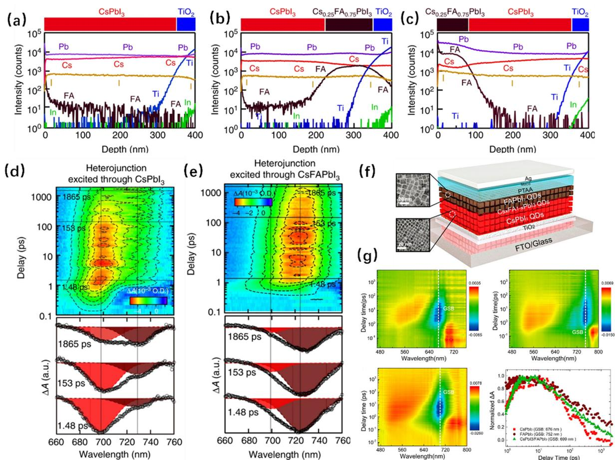
Fig. 7 (a)–(c) ToF–SIMS depth profile of samples with the structure and interface location. (d) and (e) Transient absorption of heterojunction QD films.<sup>59</sup> Copyright 2019, Springer Nature. (f) Schematic illustration of the PSCs. (g) TA measurements for time–wavelength–dependent TA color maps and TA spectra at a different GSB as a function of delay time.<sup>60</sup> Copyright 2019, American Chemical Society.
