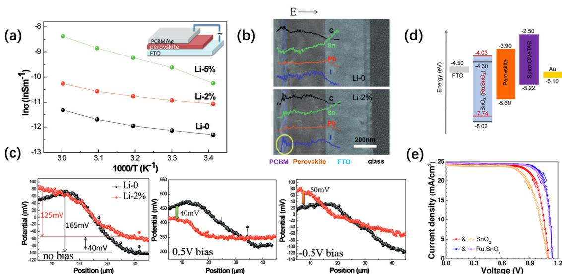
Fig. 16 (a) EDX linear scan of the element distribution. (b)  $\sigma$ - $T$  plots of Li-0, 2, and 5% in Arrhenius coordinates; the inset is the device structure. (c) The surface potential profiles (line scan) at 0 V bias, 0.5 V bias, and -0.5 V bias.<sup>113</sup> Copyright 2017, Wiley. (d) Schematic illustration of the energy level diagram of the presented PSCs. (e) Hysteresis curves.<sup>114</sup> Copyright 2019, ACS.
