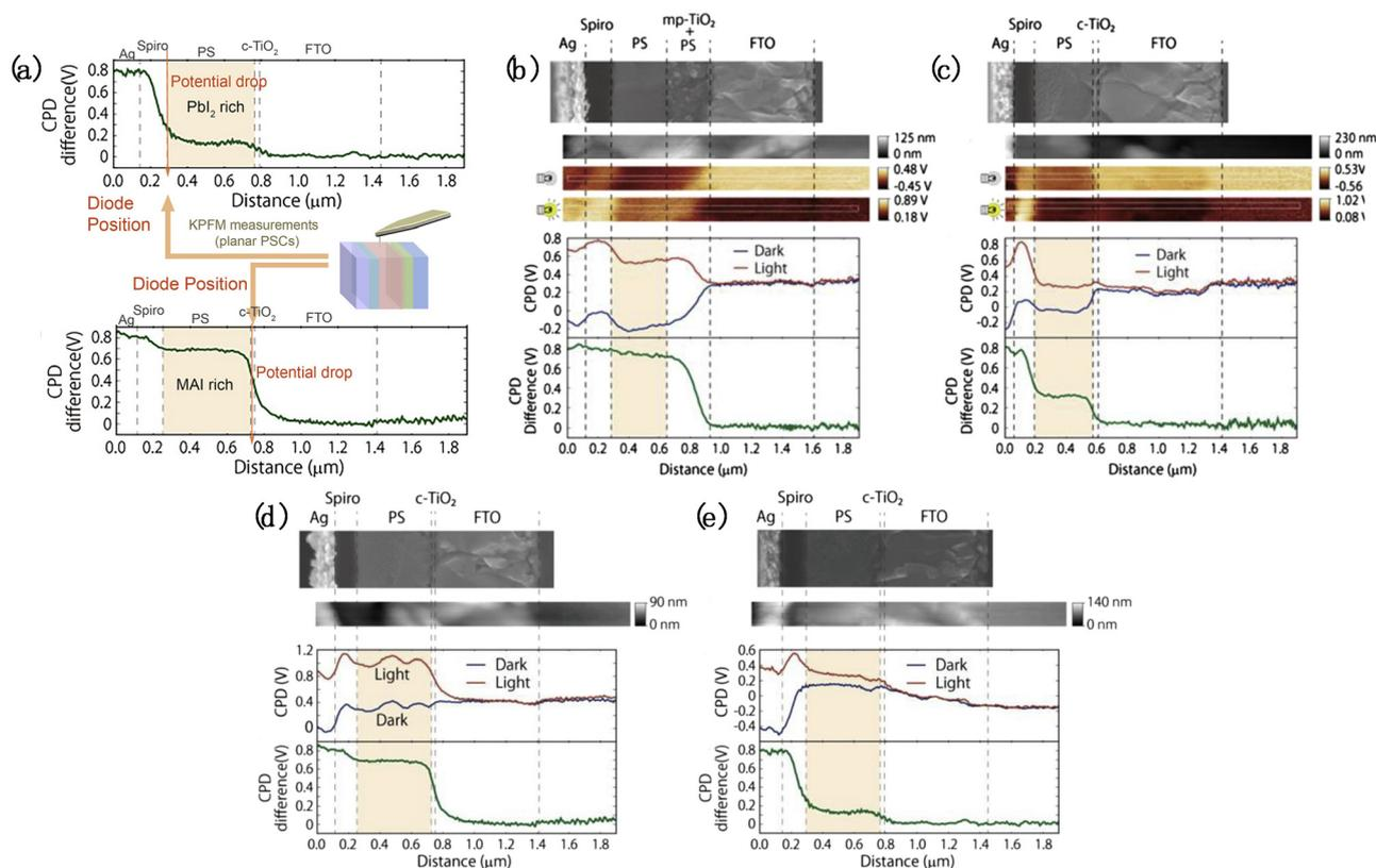
Fig. 4 (a) KPFM measurements of planar PSCs. (b) and (c) KPFM characterization of the mesoporous type PSCs fabricated using MAI- and  $\text{PbI}_2$ -rich precursors. (d) and (e) KPFM characterization of the planar type PSCs fabricated using MAI- and  $\text{PbI}_2$ -rich precursors.<sup>44</sup> Copyright 2018, Elsevier.
