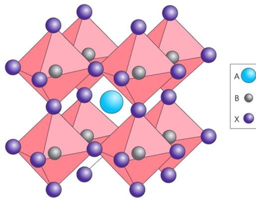
Fig. 5 Cubic perovskite crystal structure.<sup>52</sup> Copyright 2014, Springer Nature.
