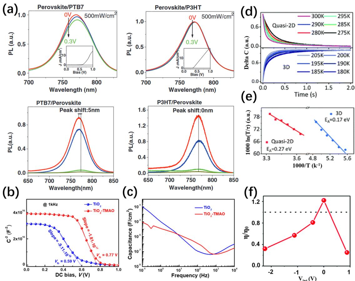
Fig. 21 (a) Electric field-induced photoluminescence spectroscopy.<sup>170</sup> Copyright 2017, Wiley. (b) Mott-Schottky analysis. (c)  $C-F$  plots. (d) Capacitance transients from anion migration (drift).<sup>171</sup> Copyright 2019, ACS. (e) Arrhenius fitting results of anion migration. (f) The function of the thermal-electrical poling voltage.<sup>173</sup> Copyright 2022, RSC.
