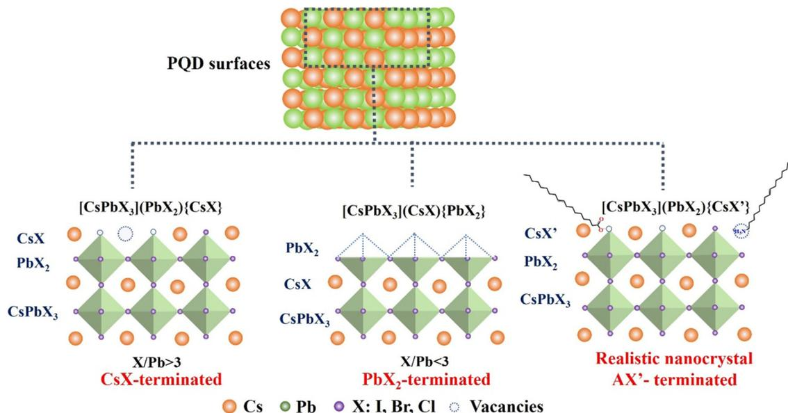
Fig. 4 Idealized surface termination models for the as-synthesized CsPbX<sub>3</sub> QDs.
