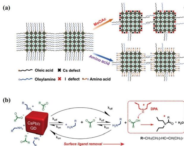
**Fig. 14** (a) Schematic illustration of the changes on the PQD surface with conventional MeOAc rinsing and dual-passivation ligands before and after ligand exchange. Reproduced with permission from ref. 141. Copyright 2020, Wiley-VCH. (b) Schematic representation of the PQD dynamic surface stabilization and the ligand removal process assisted by DPA. Reproduced with permission from ref. 142. Copyright 2020, Wiley-VCH.
