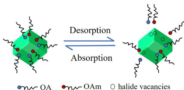
Fig. 5 Schematic representation of the dynamic surface stabilization in CsPbX<sub>3</sub> QDs.
