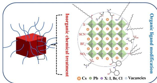
Fig. 6 Schematic illustration of the ligand-capped PQDs and an enlarged view of the nanocrystal surface with defects and different types of surface ligands used for the stabilization of PQDs.
