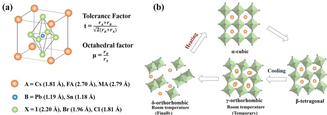
Fig. 1 (a) A cubic perovskite crystal structure ( $\alpha$ -phase) showing flexibility in the choice of cation (A), metal (B), and anion (X), whose ionic radii are shown. (b) Schematic presentation of the structural phase transition of various polymorphs of CsPbI<sub>3</sub> as a function of temperature.
