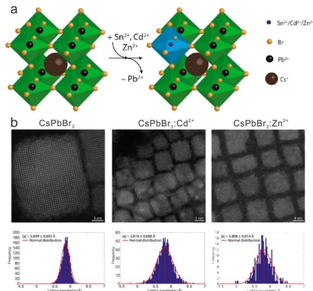
Fig. 5 (a) Schematic illustration of partial cation exchange of host Pb<sup>2+</sup> with guest M<sup>2+</sup> ions (M = Mn, Zn and Cd) in CsPbBr<sub>3</sub> NCs. (b) Quantitative high-angle annular dark-field STEM images of CsPbBr<sub>3</sub>, CsPbBr<sub>3</sub>:Cd<sup>2+</sup> and CsPbBr<sub>3</sub>:Zn<sup>2+</sup>. Reproduced with permission from ref. 99. Copyright 2017, American Chemical Society.
