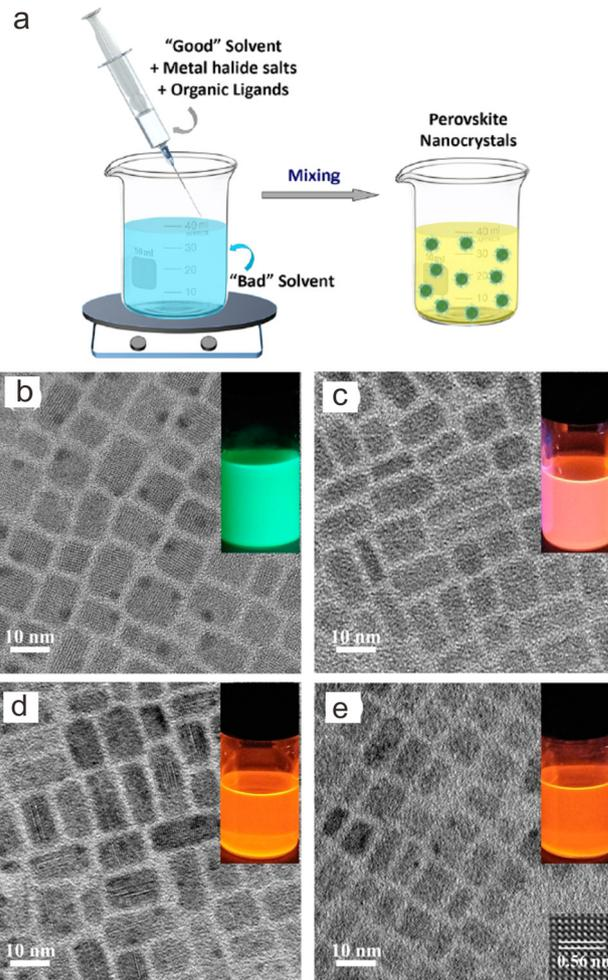
**Fig. 6** (a) Schematic illustration of supersaturated crystallization method. TEM images of (b)  $\text{CsPbBr}_3$  NCs and  $\text{CsPb}(\text{Cl}/\text{Br})_3:\text{Mn}^{2+}$  NCs with Mn/Pb molar feed ratios of (c) 2.0, (d) 5.0, and (e) 7.5, respectively. Insets show their PL photographs dispersed in cyclohexane under ultraviolet lamp irradiation. Reproduced with permission from ref. 52. Copyright 2017, American Chemical Society.
