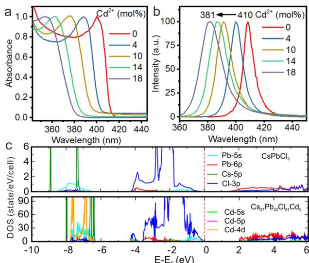
Fig. 9 (a) Absorption and (b) PL spectra for the pure CsPbCl<sub>3</sub> and CsPbCl<sub>3</sub>:Cd<sup>2+</sup> NCs. (c) Calculated density of states for pure CsPbCl<sub>3</sub> and CsPbCl<sub>3</sub>:Cd<sup>2+</sup>. Reproduced with permission from ref. 89. Copyright 2021, Wiley-VCH Verlag GmbH & Co. KGaA, Weinheim.
