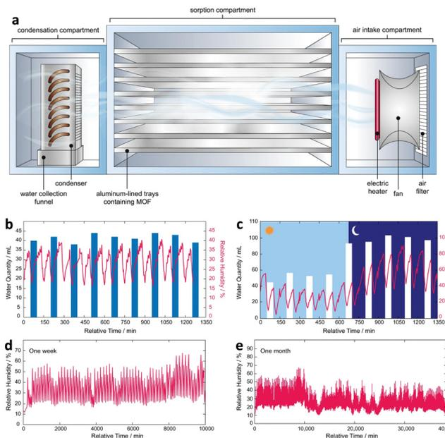
Fig. 13 (a) Schematic of the atmospheric water harvester. (b) Stress test for 24 h performed under a controlled environment (20% RH and  $25^\circ\text{C}$ ). (c) Assessment of real-world performance over a full day. (d) Real-environment continuous performance for one week. (e) Performance of self-adaptive water harvesting devices during continuous operation for a month. Reproduced with permission from ref. 109. Copyright 2022, The Author(s).
