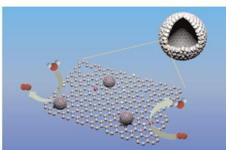
**Zeolitic imidazolite framework derived bifunctional N,P-codoped hollow carbon sphere electrocatalysts decorated with  $\text{Co}_2\text{P}/\text{Fe}$  for rechargeable Zn–air batteries**
