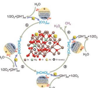
**Au depositing and Mg doping synergistically regulates an  $\text{In}_2\text{O}_3$  photocatalyst for promoting  $\text{CO}_2$  reduction and  $\text{CH}_4$  exclusive generation**
