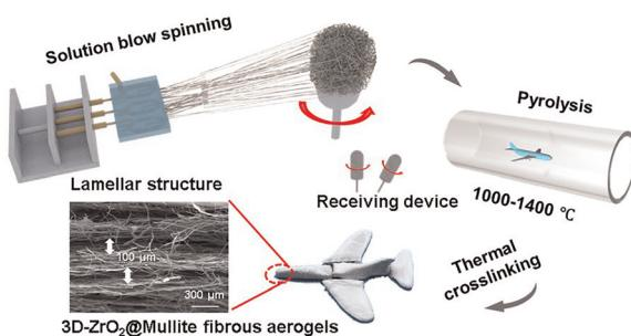
**Solution blow spinning of elastic 3D complex  $\text{ZrO}_2$ @mullite nanofibrous aerogels toward customized thermal insulation**
