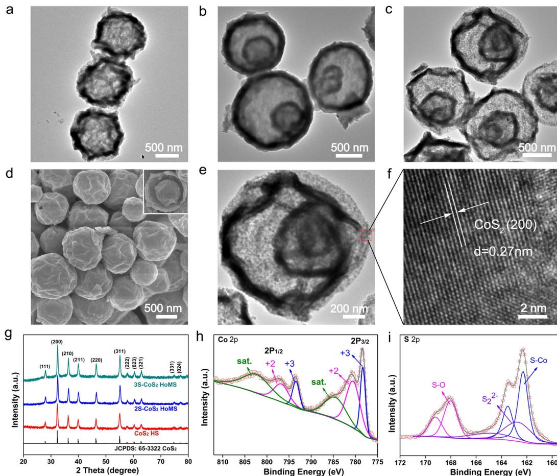
**Fig. 1** The composition and structural characterization of  $\text{CoS}_2$  HoMS. TEM images of the (a) single (1S-), (b) double (2S-), and (c) triple (3S-) shelled  $\text{CoS}_2$  HoMS. (d) SEM image of 3S- $\text{CoS}_2$  HoMS with an inset image of a broken sphere showing the multishelled structure. (e) TEM and (f) HRTEM images of an individual 3S- $\text{CoS}_2$  HoMS. (g) XRD patterns of the as-prepared samples. (h and i) XPS spectra of the Co 2p peaks (h) and S 2p peaks (i).
