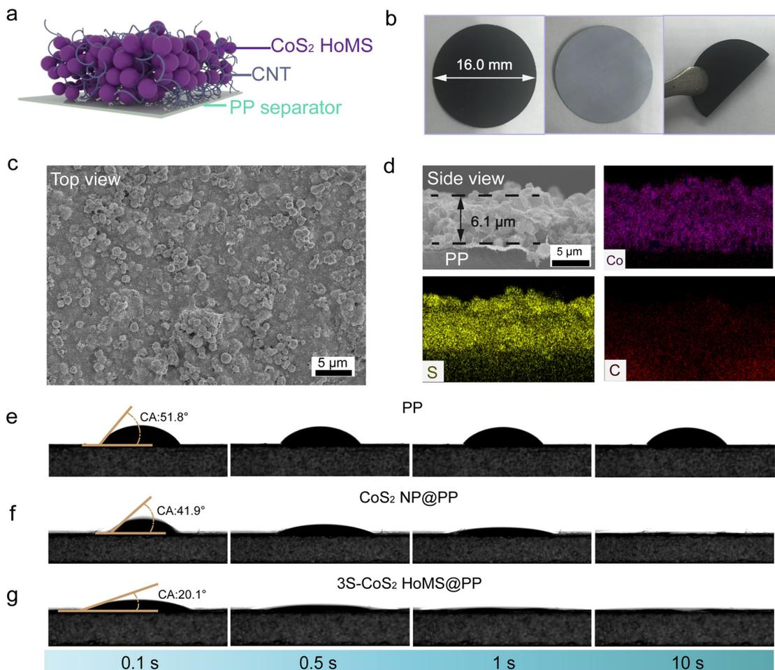
**Fig. 2** The morphology and wettability characterization of different separators. (a) Schematic diagram of the  $\text{CoS}_2$  HoMS-coated separator. (b) Optical photographs, (c) top-view, and (d) cross-section SEM images of the 3S- $\text{CoS}_2$  HoMS-coated separator. (e–g) Comparison of the contact angles of PP (e),  $\text{CoS}_2$  NP (f) and 3S- $\text{CoS}_2$  HoMS (g) coated separator at different contact times.
