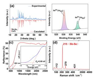
Fig. 4 (a) PXRD patterns of CBSS; (b) XPS spectrum of the CBSS sample; (c) UV-vis-NIR diffuse spectrum and experiment band gap; and (d) the Raman spectrum of CBSS.
