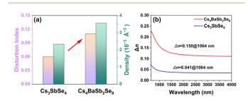
Fig. 6 (a) Comparison of the tetrahedral distortion index and functional unit density between CSS and CBSS; and (b) the calculated birefringence of CSS and CBSS.
