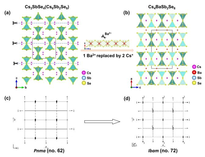
Fig. 3 (a and b) Structural evolution from (a) Cs<sub>3</sub>SbSe<sub>4</sub> to (b) Cs<sub>4</sub>BaSb<sub>2</sub>Se<sub>8</sub> based on an aliovalent-cation-substitution-induced strategy; and (c and d) the spatial symmetry operation change from CSS [low symmetry Pnma (no. 62)] to CBSS [high symmetry Ibam (no. 72)].
