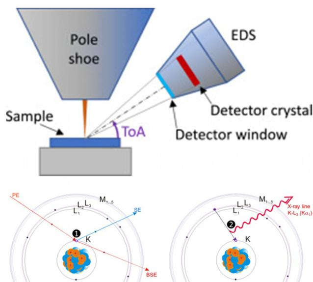
Fig. 10 Schematic system of the SEM-EDS equipment and the process of the emission of characteristic X-rays.<sup>83</sup> Copyright 2020 Elsevier.
