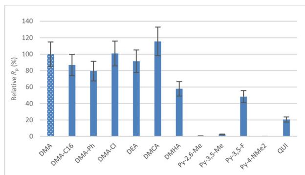
**Fig. 5** Relative productivities with respect to that with **AlHAI\_DMA** obtained with **Cat-Zr** at  $B/Zr = 100$  in combination with various AAB cocatalysts (see Table 3). 15% experimental uncertainty is assumed on  $R_p$ .
