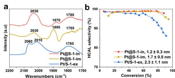
**Fig. 4** Investigation of the effect of Pt particle size on the HCAL selectivity. (a) FTIR spectra of CO chemisorbed onto the Pt/S-1-ex, Pt@S-1-im, and Pt@S-1-in catalysts at room temperature. Spectra are offset for clarity. (b) HCAL selectivity plotted against CAL conversion on catalysts with small (Pt@S-1-in), medium (Pt@S-1-im), and large (Pt/S-1-ex) Pt particles.
