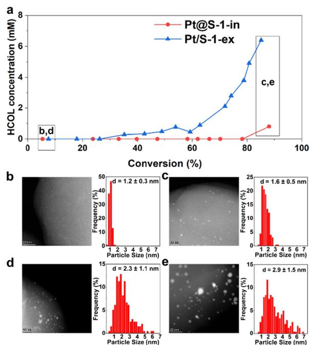
**Fig. 5** Evolution of particle size with reaction progression and the resulting effect on selectivity. (a) Concentration of hydrocinnamyl alcohol (HCOL) produced versus conversion of 83 mM cinnamaldehyde over Pt@S-1-in and Pt/S-1-ex catalysts. HAADF-STEM images and particle size distributions prior to the reaction and after ~85% cinnamaldehyde (CAL) conversion of (b and c) Pt@S-1-in at 0 and 48 h TOS, and (d and e) of Pt/S-1-ex at 0 and 72 h TOS.
