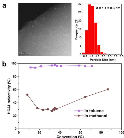
**Fig. 3** (a) HAADF-STEM image and particle size distribution of Pt@S-1-in catalyst used to study the effect of solvent polarity on Hydrocinnamaldehyde (HCAL) selectivity. (b) HCAL selectivity plotted as a function of conversion on Pt@S-1-in-l with toluene as a solvent at 100 °C or methanol as a solvent at 60 °C using similar conditions to those reported by Zhang *et al.*<sup>20</sup>
