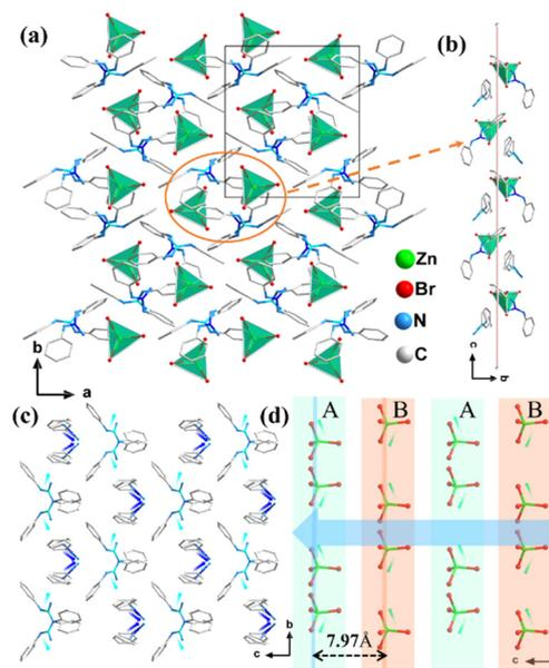
**Fig. 1** (a) The structure of **1** along the  $c$ -axis; (b) the inorganic and organic parts rotating along the  $c$  axis with  $pseudo\text{-}2_1$  helical arrangement; (c) the organic layers parallel with the  $ac$  plane; (d) the inorganic layers in the  $bc$  plane and their distance. Hydrogen atoms are omitted for clarity.
