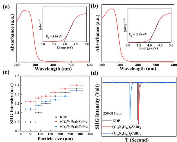
**Fig. 2** UV-vis absorption spectra and the optical band gaps obtained from Tauc plots (inset) of (a) **1** and (b) **2**; (c) particle size-dependent SHG intensity of **1**, **2** and KDP at 1064 nm; (d) SHG intensity of **1**, **2** and KDP at particle sizes of 250–315  $\mu\text{m}$ .
