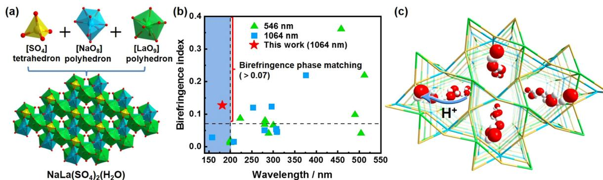
**Scheme 1** (a) Synthesis of  $\text{NaLa}(\text{SO}_4)_2(\text{H}_2\text{O})$  using a complementary cation strategy. (b) Comparison of birefringence with the literature.<sup>11,18,21–35</sup> (c) 1D spiral water chain promoted high proton conductivity of  $\text{NaLa}(\text{SO}_4)_2(\text{H}_2\text{O})$ .
