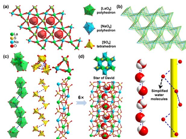
**Fig. 1** Crystal structure of  $\text{NaLa}(\text{SO}_4)_2(\text{H}_2\text{O})$ . (a) Simplified *sma* topology. (b) View of the framework along the *c* axis. (c) 1D triangular prism  $[\text{NaLa}(\text{SO}_4)_2]_\infty$  (right), and packing manners of  $[\text{LaO}_9]$  polyhedron (left) and  $[\text{SO}_4]$  tetrahedron (middle). (d) Structure of 1D pore (nanotube, left) and spiral water chain in the nanotube (right).
