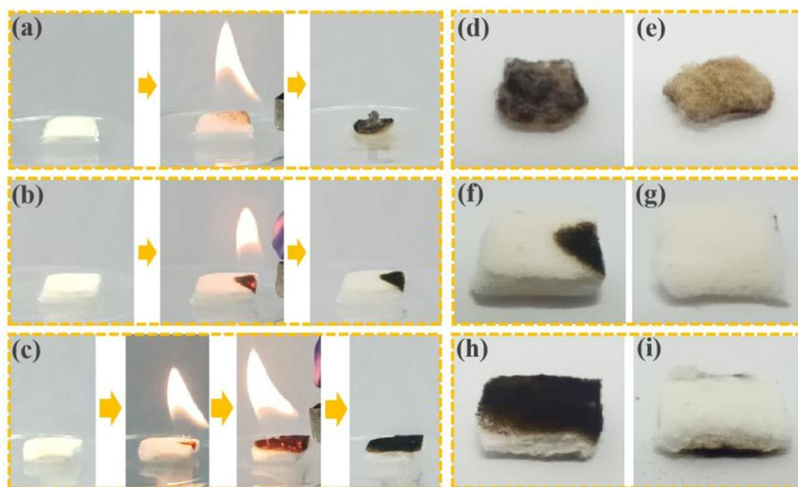
**Fig. 4** Burning state of cotton kindling (a) and 2CF<sub>3</sub>-UiO-66@CT igniting part (b) and igniting whole side (c); the morphology of 2CF<sub>3</sub>-UiO-66@CT ignition surface and unignited surface of cotton (d and e) and combustion part (f and g) and combustion whole side (h and i).
