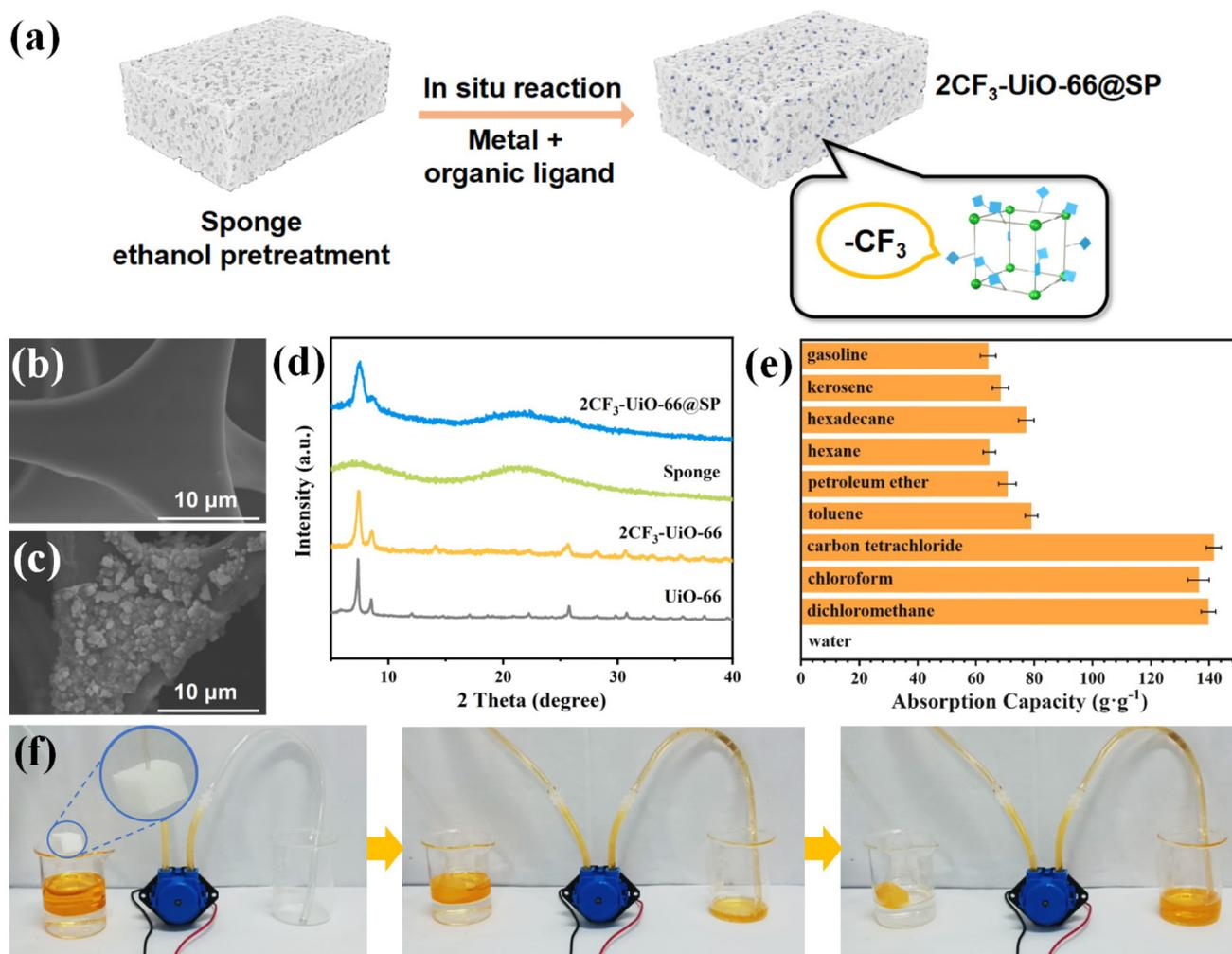
**Fig. 5** (a) Schematic representation of the synthesis of  $2CF_3\text{-UiO-66@SP}$  (b) SEM image of sponge. (c) SEM image of  $2CF_3\text{-UiO-66@SP}$ . (d) PXRD experimental data of  $2CF_3\text{-UiO-66@SP}$ , sponge,  $2CF_3\text{-UiO-66}$ , and UiO-66. (e) The adsorption capacity of  $2CF_3\text{-UiO-66@SP}$  for different solvents. (f) Images of automatic light oil (dyed with Sudan I) adsorption device and its separation process using  $2CF_3\text{-UiO-66@SP}$ .
