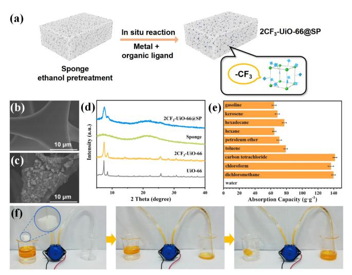
Fig. 5 (a) Schematic representation of the synthesis of 2CF<sub>3</sub>-UiO-66@SP (b) SEM image of sponge. (c) SEM image of 2CF<sub>3</sub>-UiO-66@SP. (d) PXRD experimental data of 2CF3-UiO-66@SP, sponge, 2CF3-UiO-66, and UiO-66. (e) The adsorption capacity of 2CF3-UiO-66@SP for different solvents. (f) Images of automatic light oil (dyed with Sudan I) adsorption device and its separation process using 2CF<sub>3</sub>-UiO-66@SP.
