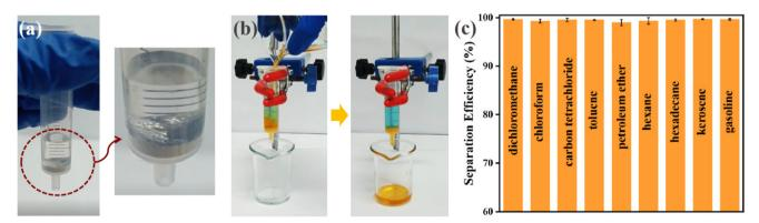
Fig. 3 (a) Images of 2CF<sub>3</sub>-UiO-66@CT separation device after adding 1 mL of deionized water (b) images of oil-water separation process using 2CF<sub>3</sub>-UiO-66@CT. Organic solvent (4 mL, containing 10 mM of Sudan I indicator for visualization) was mixed with deionized water (3 mL). The organic solvent could pass through 2CF<sub>3</sub>-UiO-66@CT while water was trapped. (c) The separation efficiency of different organic solvents and water using 2CF<sub>3</sub>-UiO-66@CT.
