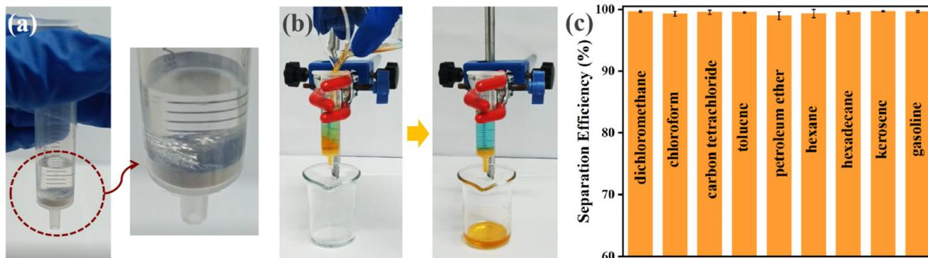
**Fig. 3** (a) Images of  $2CF_3$ -UiO-66@CT separation device after adding 1 mL of deionized water (b) images of oil–water separation process using  $2CF_3$ -UiO-66@CT. Organic solvent (4 mL, containing 10 mM of Sudan I indicator for visualization) was mixed with deionized water (3 mL). The organic solvent could pass through  $2CF_3$ -UiO-66@CT while water was trapped. (c) The separation efficiency of different organic solvents and water using  $2CF_3$ -UiO-66@CT.
