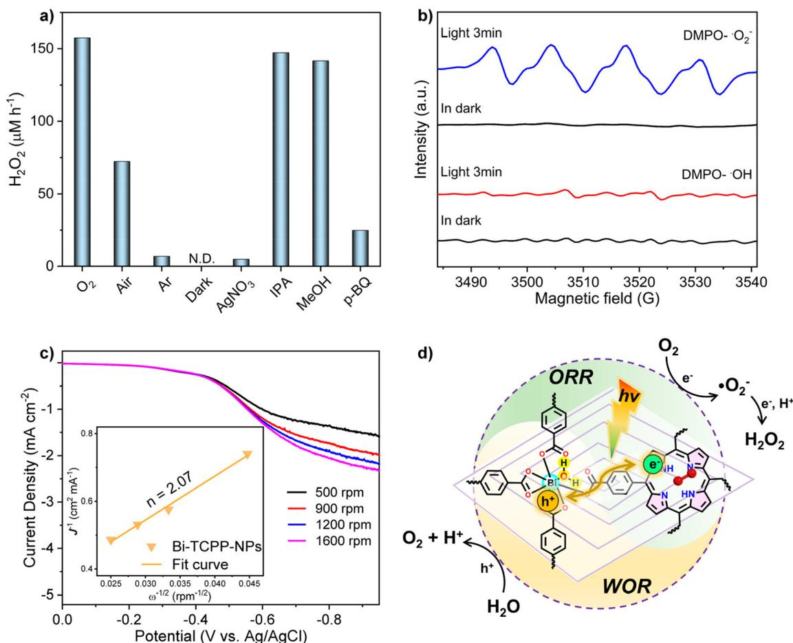
**Fig. 5** (a) The photocatalytic  $\text{H}_2\text{O}_2$  production rates with different scavengers and atmospheres. (b) EPR spectra of Bi-TCPP-NPs. (c) The Koutecky–Levich plots obtained by RDE measurements at  $-0.80 \text{ V}$  vs.  $\text{Ag}/\text{AgCl}$ . (d) The proposed mechanistic catalytic diagrams over Bi-TCPP-NPs.
