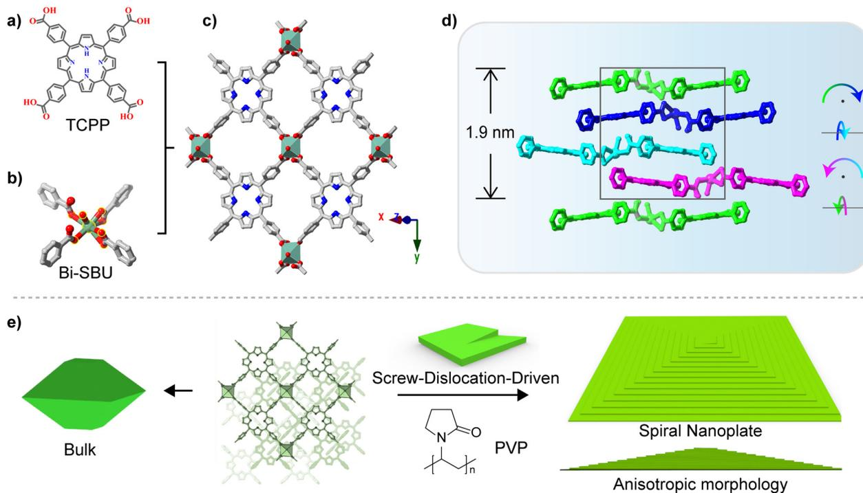
**Fig. 1** (a–c) Structure of Bi-TCPP and its assembly units, viz. Bi-carboxylate node and TCPP linker. (d) Side-view of the stacking mode of 2D layers in Bi-TCPP along the *b*-axis. (e) Diagram of growth mechanism for Bi-TCPP-bulk and Bi-TCPP-NPs.
