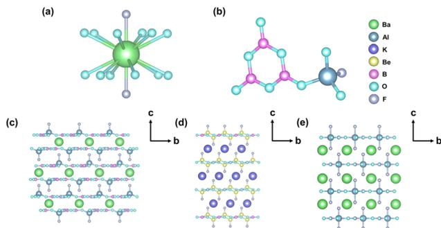
**Fig. 2** (a) The coordination environment of the Ba atom. (b) The basic building block of  $[\text{AlB}_3\text{O}_6\text{F}]$  formed by the connection of  $[\text{B}_3\text{O}_6]$  and  $[\text{AlO}_3\text{F}]$  groups. Crystal structures of (c)  $\text{BaAl}_2(\text{B}_3\text{O}_6)_2\text{F}_2$ , (d)  $\text{KBe}_2\text{B}_3\text{O}_3\text{F}_2$ , and (e)  $\text{BaAlBO}_3\text{F}_2$  in the  $a$  direction.
