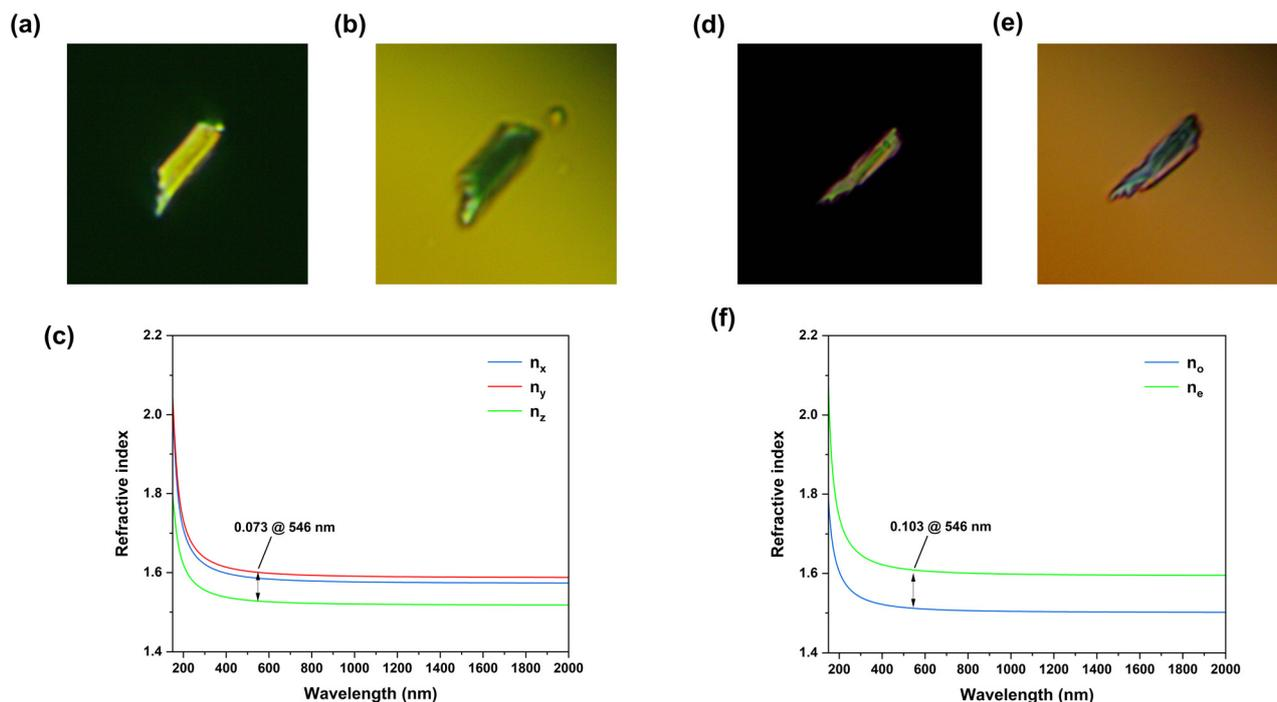
**Fig. 4** Photos of the original (a)  $\text{BaAlB}_3\text{O}_6\text{F}_2$  crystal and (d)  $\text{BaAl}_2(\text{B}_3\text{O}_6)_2\text{F}_2$  crystal. Photos of (b) the  $\text{BaAlB}_3\text{O}_6\text{F}_2$  crystal and (e) the  $\text{BaAl}_2(\text{B}_3\text{O}_6)_2\text{F}_2$  crystal after extinction. The calculated refractive indices of (c)  $\text{BaAlB}_3\text{O}_6\text{F}_2$  and (f)  $\text{BaAl}_2(\text{B}_3\text{O}_6)_2\text{F}_2$ .
