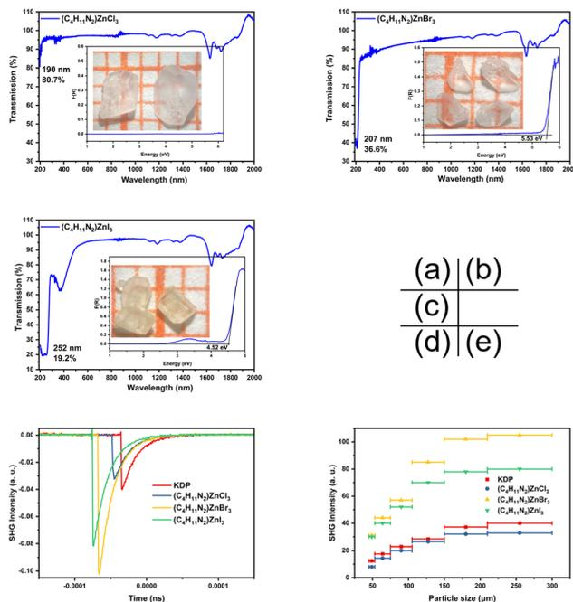
**Fig. 4** UV transmittance spectra (a, b, c for Cl, Br, and I compounds, respectively). The inset shows the bandgaps and as-grown crystals.  $F(R)$  is the absorption coefficient/scattering coefficient. Oscilloscope traces of the SHG signals (150–210  $\mu\text{m}$ ) with 1064 nm laser radiation (d) and Phase-matching curves (e). KDP was used as references for the SHG measurements.
