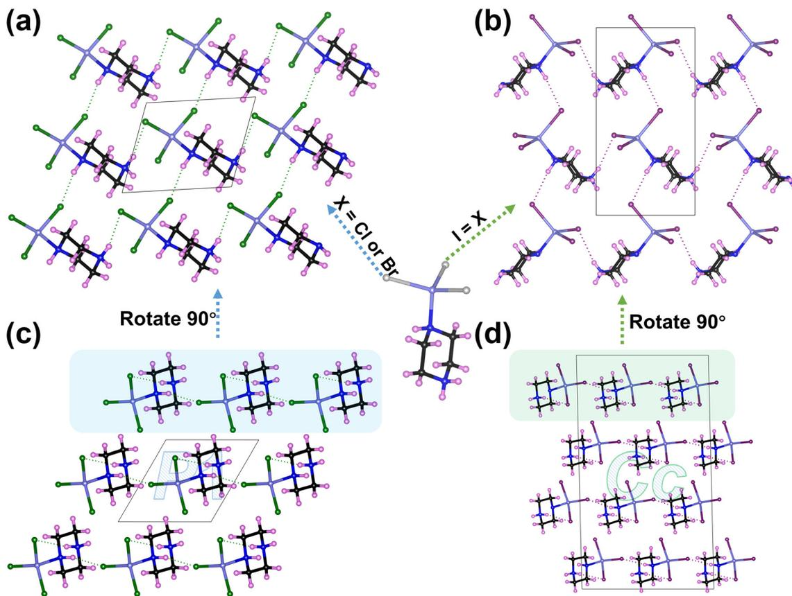
**Fig. 2** Views of the structures of 2D  $[(C_4H_{11}N_2)ZnCl_3]_{\infty}$  neutral layer along *a* direction (a), 3D  $(C_4H_{11}N_2)ZnCl_3$  along *c* direction (b), 2D  $[(C_4H_{11}N_2)ZnI_3]_{\infty}$  neutral layer along *a* direction, and 3D  $(C_4H_{11}N_2)ZnI_3$  along *b* direction (d). The spheres of pink, violet-blue, blue, black, green, and dark purple respectively represent the atoms of H, Zn, N, C, Cl, and I.
