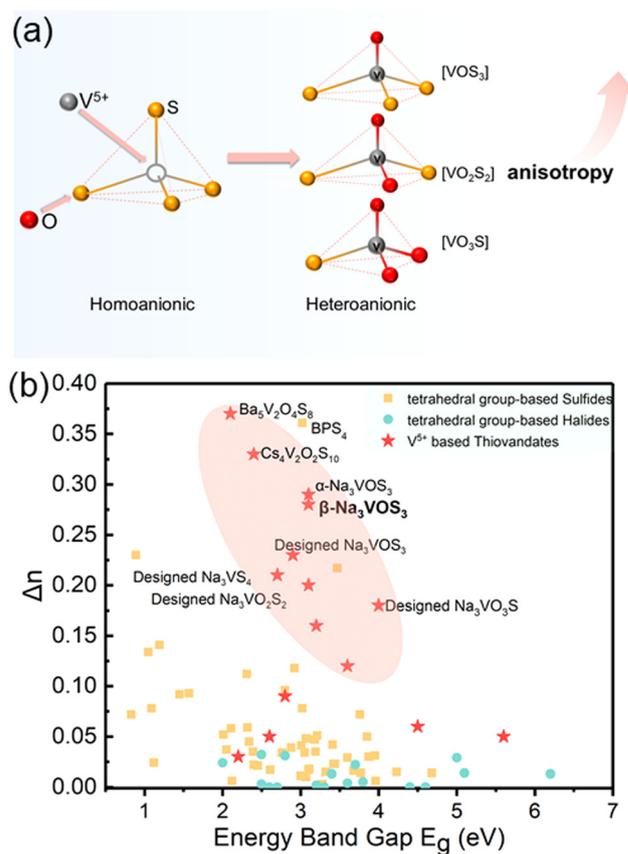
**Fig. 1** (a) Schematic of our design strategy for enlarging the birefringence of the tetrahedral group; (b) balanced performance coordinate of the  $\Delta n$  and energy band gap in the tetrahedral-based sulfides, halides and  $V^{5+}$ -based thiovanadates (the data of the tetrahedral-based sulfides and halides are from ref. 33 and 50, and compounds are listed in Table S1†).
