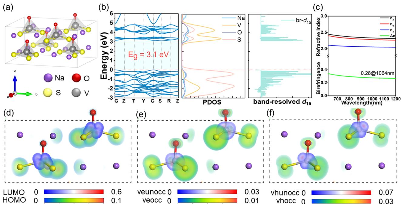
**Fig. 2** (a) Unit cell in  $\beta$ - $\text{Na}_3\text{VOS}_3$ ; (b) band structures (left panel), PDOS (middle panel) and band-resolved  $d_{15}$  (right panel); (c) dispersion curves of the refractive indices and birefringence of  $\beta$ - $\text{Na}_3\text{VOS}_3$ ; (d) HOMO and LUMO; SHG-weighted density for occupied and unoccupied (e) VE process; (f) VH process.
