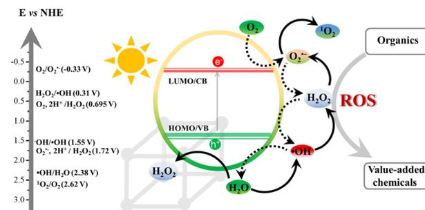
Fig. 14 General illustration of possible reactive oxygen species (ROS) in MOF-based photocatalysts responsible for oxidation reactions under an aqueous and aerobic conditions.<sup>171</sup>
