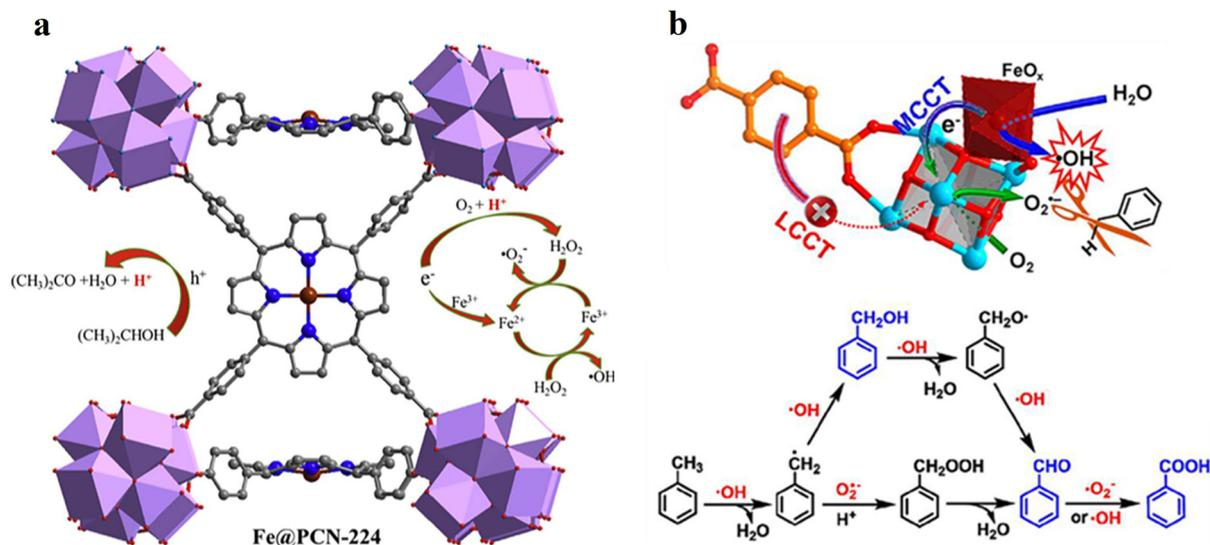
**Fig. 17** (a) Proposed mechanism of oxygen-related radical generation in photocatalytic systems with Fe@PCN-224. Adapted with permission from ref. 195. Copyright 2018, Elsevier. (b) Schematic illustration showing the conversion of H<sub>2</sub>O to •OH by visible light-driven MCCT process over Fe-doped UiO-66 and proposed catalytic mechanism of toluene oxidation. Adapted with permission from ref. 87. Copyright 2019, the American Chemical Society.
