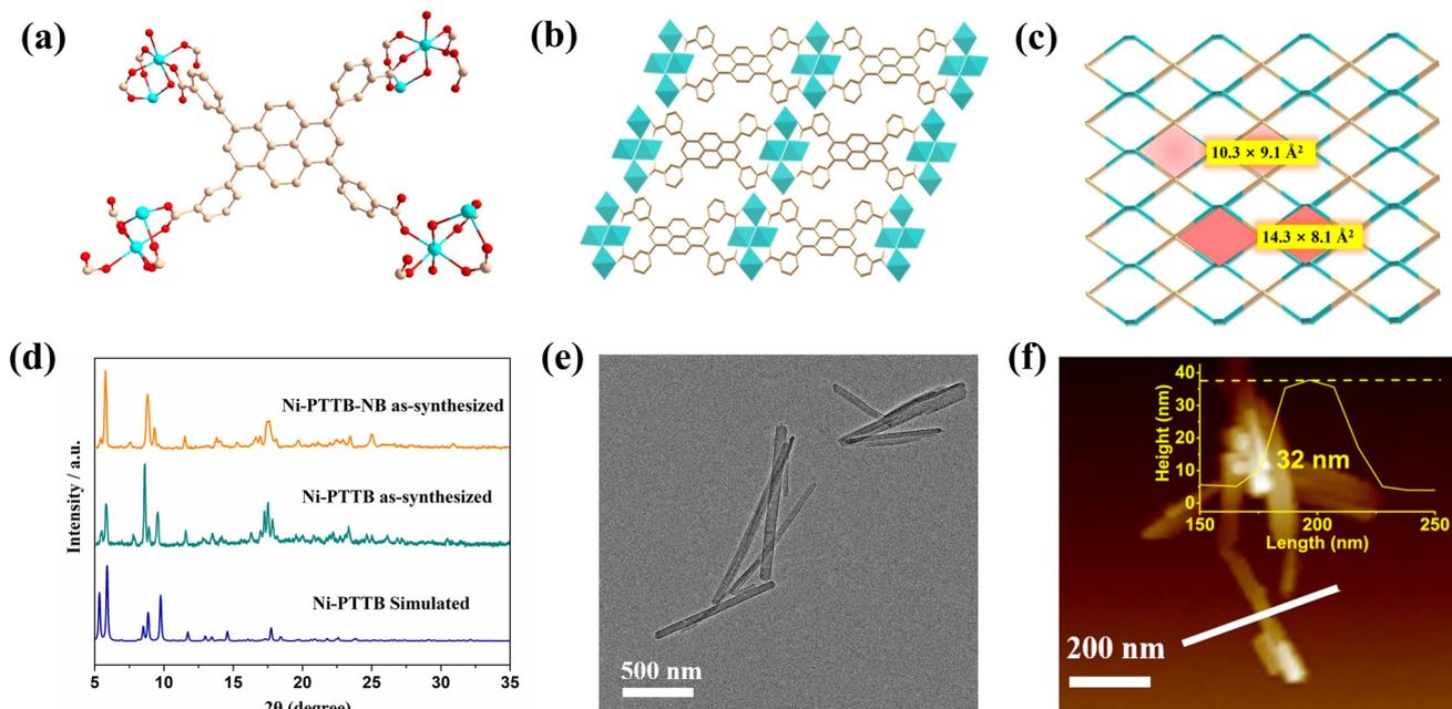
**Fig. 1** (a) Characterization of Ni-PTTB and Ni-PTTB-NB. Coordination environment of the PTTB $^{4-}$  ligand; (b) 2D layered structure viewed along the *b*-axis direction; (c) schematic representation of the (4,4)-connected framework of Ni-PTTB with the **sql** topology; (d) PXRD patterns; (e) TEM image of Ni-PTTB-NB; (f) atomic force microscopy (AFM) image of Ni-PTTB-NB (insert: height profile).
