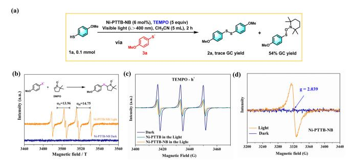
Fig. 3 (a) Trapping of thiyl radicals; (b) EPR spectrum of capturing thiyl radicals over Ni-PTTB-NB; (c) EPR spectra of TEMPO-h<sup>+</sup> over Ni-PTTB and Ni-PTTB-NB; (d) EPR spectra of Ni-PTTB-NB, manifesting the formation of Ni<sup>+</sup> during photocatalysis
