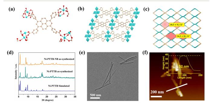
Fig. 1 (a) Characterization of Ni-PTTB and Ni-PTTB-NB. Coordination environment of the PTTB<sup>4-</sup> ligand; (b) 2D layered structure viewed along the b-axis direction; (c) schematic representation of the (4,4)-connected framework of Ni-PTTB with the sql topology; (d) PXRD patterns; (e) TEM image of Ni-PTTB-NB; (f) atomic force microscopy (AFM) image of Ni-PTTB-NB (insert: height profile).
