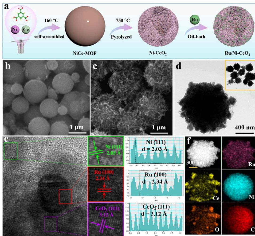
**Fig. 1** (a) Preparation diagram of Ru/Ni-CeO<sub>2</sub> catalyst. SEM images of (b) NiCe-MOF and (c) Ru/Ni-CeO<sub>2</sub>. (d) TEM image of Ru/Ni-CeO<sub>2</sub>. (e) High-resolution TEM image of Ru/Ni-CeO<sub>2</sub>. (f) Elemental mappings of Ru/Ni-CeO<sub>2</sub>.
