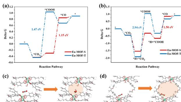
**Fig. 5** (a and b) Gibbs free energy diagram of the  $\text{CO}_2$  reduction pathway of Eu-MOFs, where in the a-figure path the proton originates from solution and in the b-figure path the proton originates from the adsorbed state  $\text{H}^+$  near the catalytic site; (c) state diagram of  $\text{CO}_2$  to  $^*\text{COOH}$  near metal sites in the pores of Eu-MOF-S; (d) state diagram of  $\text{CO}_2$  to  $^*\text{COOH}$  near metal sites in the pores of Eu-MOF-T.
