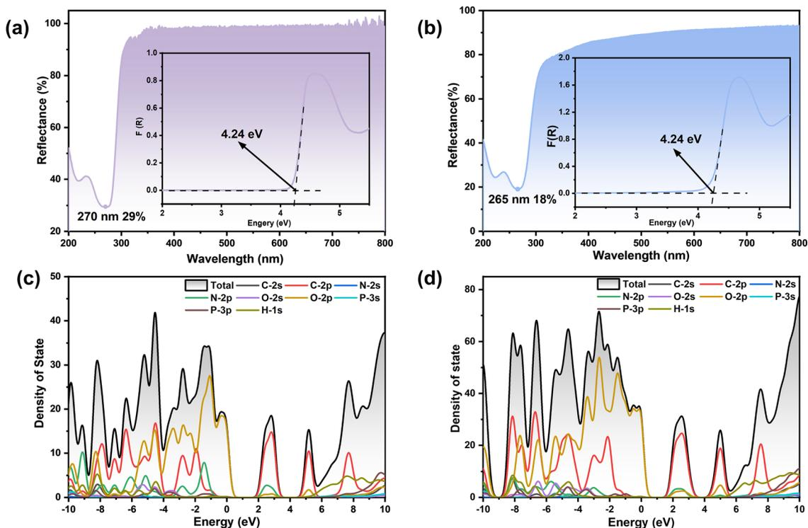
Fig. 4 UV-vis diffuse reflectance spectra (the inset show the bandgaps and  $F(R)$  is absorption coefficient/scattering coefficient.) for **I** (a) and **II** (b), as well as the density of states for **I** (c) and **II** (d).
