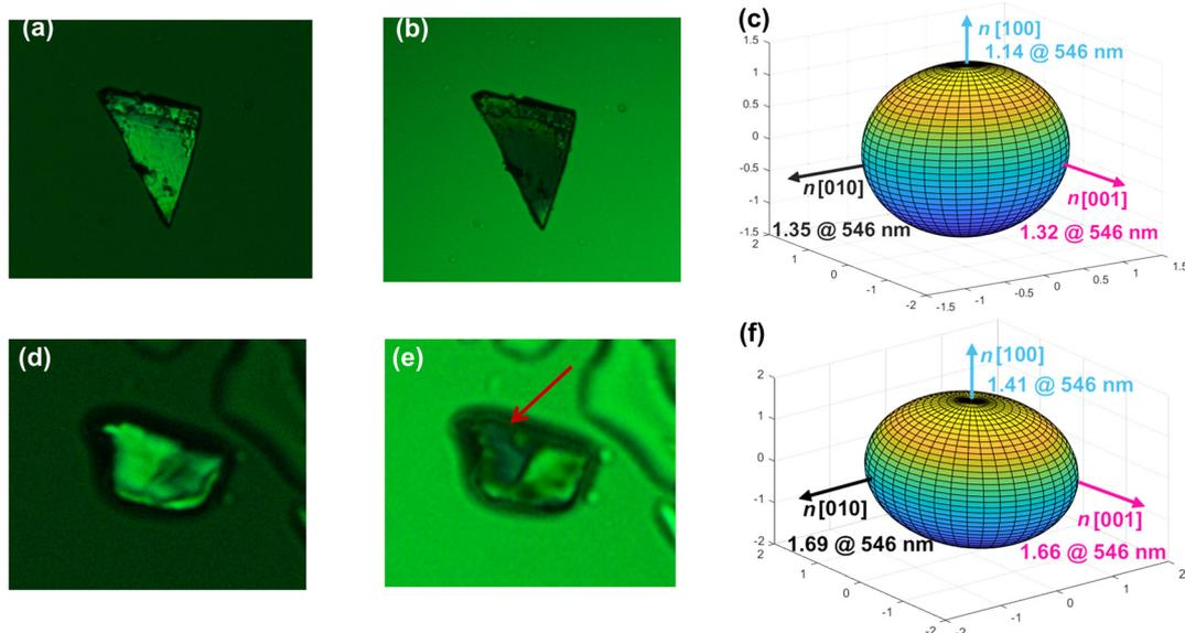
Fig. 6 Original crystal, crystals achieving complete extinction and triaxial ellipsoid of three refractive indices along crystallographic axes for **I** (a–c) and **II** (d–f).
