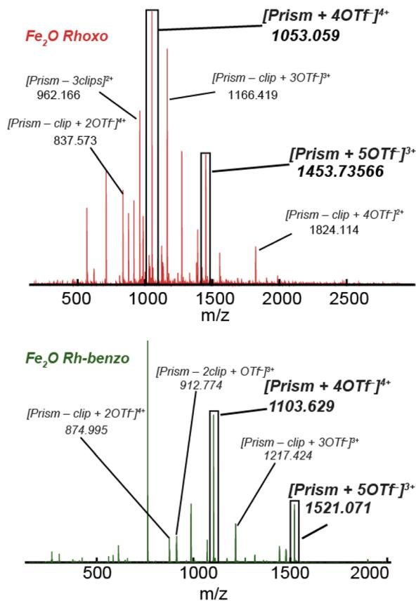
**Fig. 5** High resolution mass spectra of  $\text{Fe}_2\text{O Rhoxo}$  (top) and  $\text{Fe}_2\text{O Rh-benzo}$  (bottom). "Prism" accounts for the mass of two porphyrins and four molecular clips. The number of counterions remaining are listed for each peak. Bolded labels correspond to peaks for intact prisms while non-bolded labels refer to fragments peaks that have lost molecular clips in addition to counterions.
