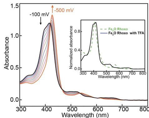
**Fig. 8** Spectroelectrochemical measurements of  $0.016 \text{ mM}$  of **Fe $_2$ O Rhoxo**,  $100 \text{ mM TBABF}_4$ ,  $100 \text{ mM TFA}$ , DMF. Initial potential:  $-100 \text{ mV}$  vs.  $\text{Ag/Ag}^+$ , final potential:  $-0.500 \text{ V}$  vs.  $\text{Ag/AgNO}_3$ . Step amplitude:  $0.050 \text{ V}$ , step period: 30 seconds. Inset: Absorbance spectra of **Fe $_2$ O Rhoxo** in DMF (green dashed) and with  $100 \text{ mM TFA}$  (black solid).
