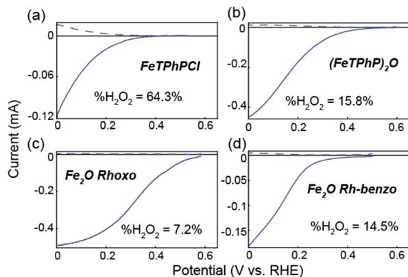
**Fig. 7** RRDE voltammograms at scan rates of  $20 \text{ mV s}^{-1}$ . In all cases, the catalysts were immobilized in Nafion inks with carbon black and immersed in  $0.5 \text{ M H}_2\text{SO}_4$ . The ring potential was held at  $1 \text{ V}$ . Scan direction: reducing. (a) **FeTPhPCI**, (b) **(FeTPhP) $_2$ O**, (c) **Fe $_2$ O Rhoxo**, (d) **Fe $_2$ O Rh-benzo**.
