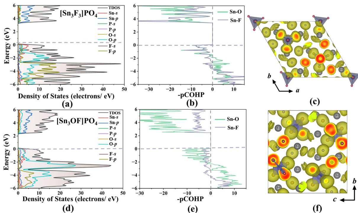
**Fig. 3** (a and d) Partial density of states (PDOS), (b and e) negative crystal orbital Hamiltonian population ( $-\text{pCOHP}$ ), and (c and f) electron localization function (ELF) diagrams of  $[\text{Sn}_3\text{F}_3]\text{PO}_4$  and  $[\text{Sn}_3\text{OF}]\text{PO}_4$ , respectively.
