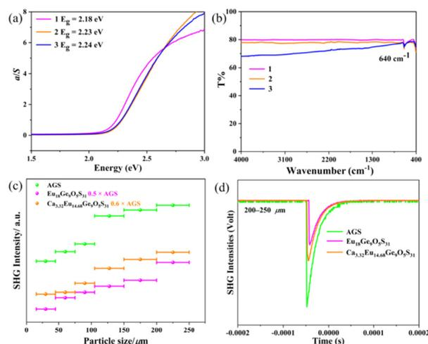
**Fig. 2** (a) The UV-vis-NIR diffuse reflection and (b) IR spectra of **1–3**; (c) size-dependent SHG responses and (d) SHG intensities at 200–250 μm of **1**, **2** and AGS under 2.1 μm laser radiation.
