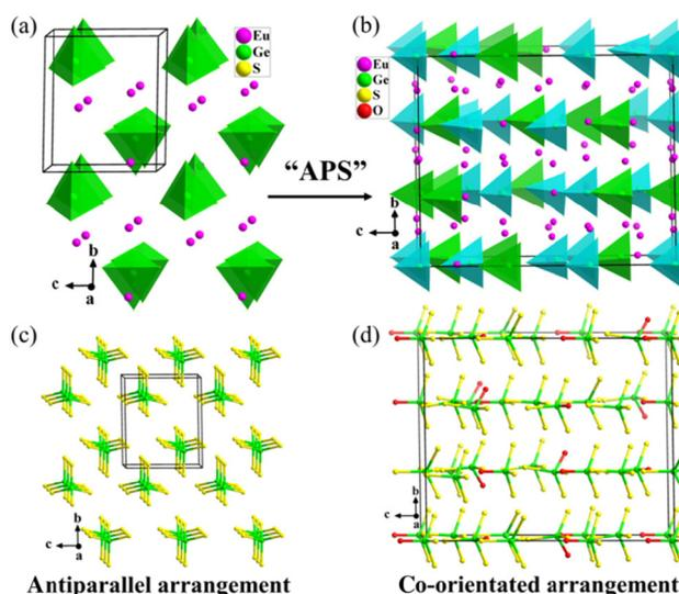
**Fig. 1** Crystal structures of **0** (a) and **1** (b); blue and green tetrahedra represent  $\text{GeOS}_3$  and  $\text{GeS}_4$  units, respectively; (c) alignment of  $\text{GeS}_4$  tetrahedra in **0**; (d) alignment of  $\text{GeS}_4$  and  $\text{GeOS}_3$  tetrahedra in **1**. The Eu–S and Eu–O bonds are omitted for clarity.
