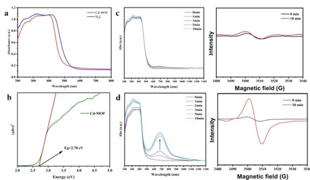
**Fig. 11** (a and b) UV-visible diffuse reflectance spectra and the Tauc plot of the Cd-MOF; (c and d) UV-visible diffuse reflectance spectra and EPR spectra of  $H_4L$  and the Cd-MOF with irradiation time.
