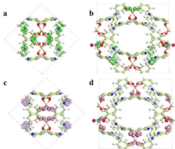
**Fig. 7** CB and VB of the Cd-MOF (a and c) and the UO<sub>2</sub><sup>2+</sup>@Cd-MOF (b and d).
