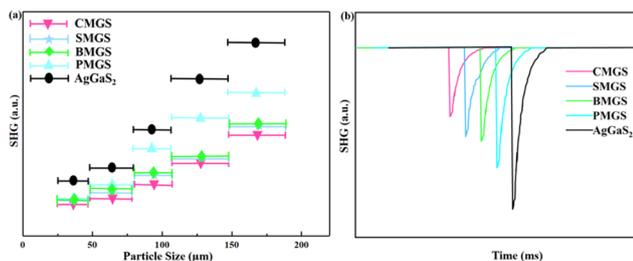
**Fig. 4** (a) Phase-matching results of  $\text{MMn}_6\text{Ga}_6\text{S}_{16}$  ( $M = \text{Ca}, \text{Sr}, \text{Ba},$  and  $\text{Pb}$ ) and the benchmark AGS at 2090 nm and (b) SHG intensities of  $\text{MMn}_6\text{Ga}_6\text{S}_{16}$  ( $M = \text{Ca}, \text{Sr}, \text{Ba},$  and  $\text{Pb}$ ) and AGS with the particle size ranging from 150–200  $\mu\text{m}$ .
