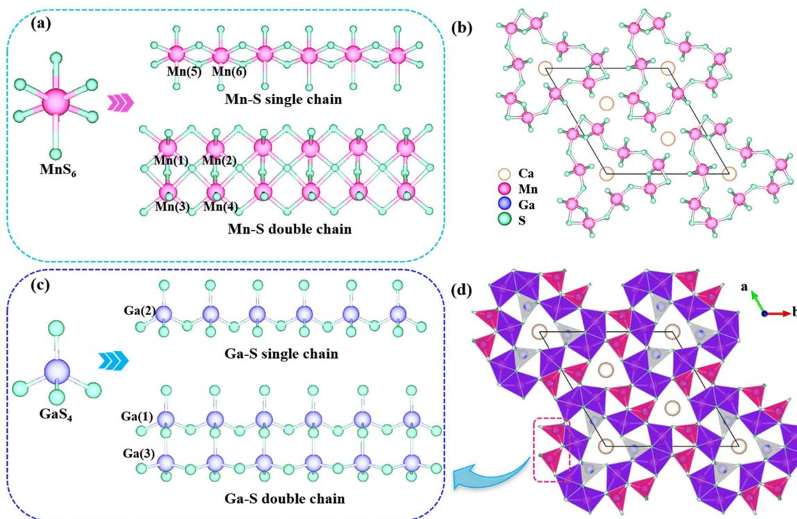
**Fig. 1** Crystal structure of CMGS: (a) MnS<sub>6</sub> octahedron and Mn-S single and double chains; (b) Mn<sub>9</sub>S<sub>39</sub> framework; (c) GaS<sub>4</sub> tetrahedron and Ga-S single and double chains; and (d) structure of CMGS viewed along the c-axis.
