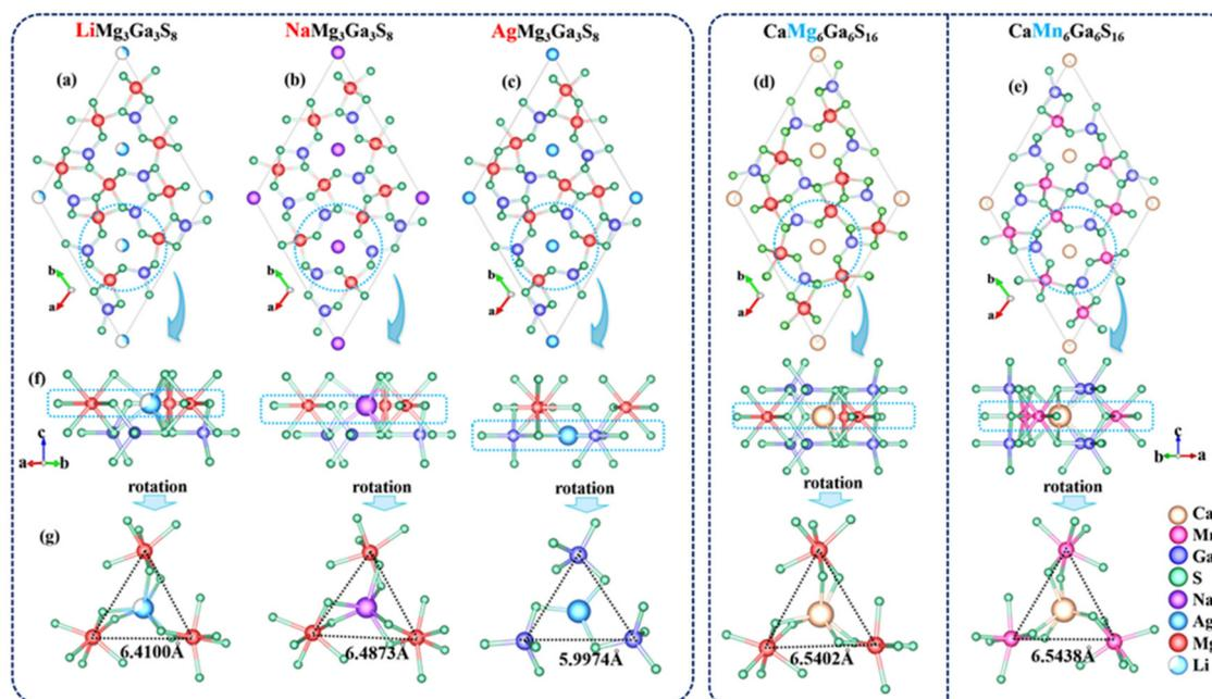
**Fig. 2** Structures of (a) LiMg<sub>3</sub>Ga<sub>3</sub>S<sub>8</sub>; (b) NaMg<sub>3</sub>Ga<sub>3</sub>S<sub>8</sub>; (c) AgMg<sub>3</sub>Ga<sub>3</sub>S<sub>8</sub>; (d) CaMg<sub>6</sub>Ga<sub>6</sub>S<sub>16</sub>; and (e) CaMn<sub>6</sub>Ga<sub>6</sub>S<sub>16</sub>; and (f and g) the location of different cations.
