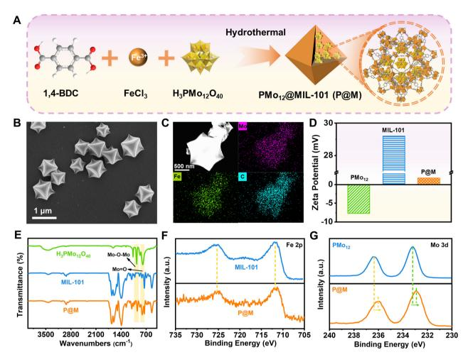
Fig. 2 Preparation and characterization of P@M. (A) Schematic illustration of the synthetic route for P@M. (B) SEM image of P@M. (C) Elemental mappings of Mo, Fe, and C signals. (D) Zeta potential of PMo<sub>12</sub>, MIL-101 and P@M. (E) FT-IR spectra of PMo<sub>12</sub>, MIL-101 and P@M. High-resolution XPS spectra of (F) Fe 2p and (G) Mo 3d for PMo<sub>12</sub> and P@M.
