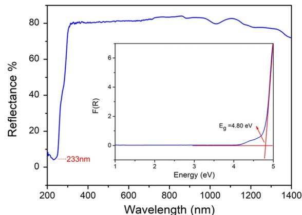
**Fig. 6** The UV-vis-NIR diffuse reflectance spectrum of MELSC.
