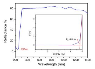
Fig. 6 The UV-vis-NIR diffuse reflectance spectrum of MELSC.
