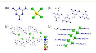
Fig. 2 Crystal structure of MELBF. (a) Basic constituent units [C<sub>3</sub>N<sub>6</sub>H<sub>7</sub>]<sup>+</sup> and  $[BF_4]^-$ . (b) The one-dimensional chain formed by  $[C_3N_6H_7]^+$  groups. (c) The two-dimensional structure formed by  $[C_3N_6H_7]^+$  and  $[BF_4]^$ groups. (d) Three-dimensional structure.
