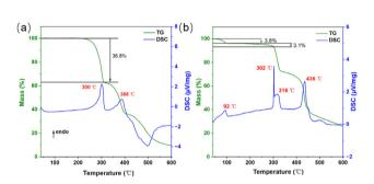
Fig. 4 The TG-DSC curves for (a) MELBF and (b) MELSC.
