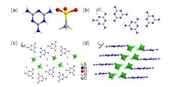
Fig. 3 Crystal structure of MELSC. (a) Basic constituent units [C<sub>3</sub>N<sub>6</sub>H<sub>7</sub>]<sup>+</sup> and  $[SO_3CH_3]^-$ . (b) The one-dimensional chain formed by  $[C_3N_6H_7]^+$ groups. (c) The two-dimensional structure of  $[C_3N_6H_7]^+$  and  $[SO_3CH_3]^$ groups. (d) Three-dimensional structural drawings.
