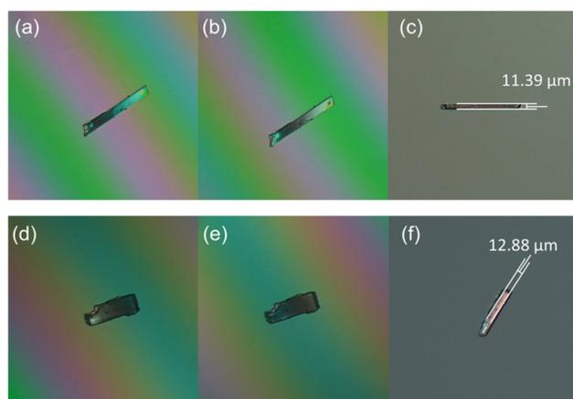
**Fig. 8** Refractive index difference measurements for **MELBF** and **MELSC**. **MELBF** single crystal under the (a) positive (up) and (b) negative (down) compensatory rotation; **MELSC** single crystal under the (d) positive (up) and (e) negative (down) compensatory rotation; (c) and (f) the thickness of **MELBF** and **MELSC**.
