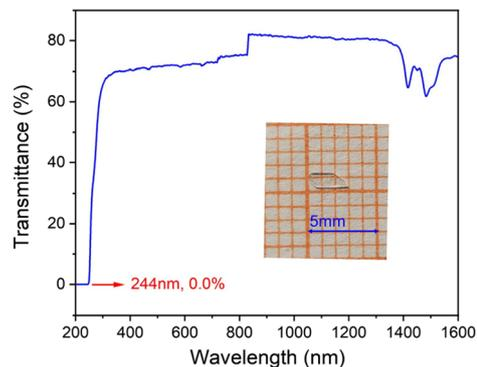
**Fig. 5** The UV-vis-NIR transmission spectrum of MELBF.
