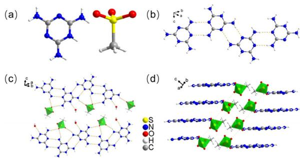
**Fig. 3** Crystal structure of MELSC. (a) Basic constituent units  $[\text{C}_3\text{N}_6\text{H}_7]^+$  and  $[\text{SO}_3\text{CH}_3]^-$ . (b) The one-dimensional chain formed by  $[\text{C}_3\text{N}_6\text{H}_7]^+$  groups. (c) The two-dimensional structure of  $[\text{C}_3\text{N}_6\text{H}_7]^+$  and  $[\text{SO}_3\text{CH}_3]^-$  groups. (d) Three-dimensional structural drawings.
