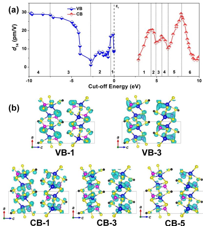
**Fig. 6** Theoretical analysis of the intrinsic mechanism of SHG source for PbPbPS<sub>4</sub>: (a) cut-off energy (eV) dependence of the static  $d_{14}$  ( $\text{pm V}^{-1}$ ); (b) distribution of the partial charge density maps with major contributions in the VB-1, VB-3, CB-1, CB-3 and CB-5 regions. Black atoms: Rb; blue atoms: Pb; pink atoms: P; yellow atoms: S.
