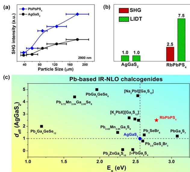
**Fig. 4** (a) SHG intensities vs. particle size at  $\lambda = 2900$  nm for PbPbPS<sub>4</sub> and AgGaS<sub>2</sub>; (b) the relative SHG and LIDT intensities of PbPbPS<sub>4</sub> and reference commercial material AgGaS<sub>2</sub> in the particle size of 150–210  $\mu\text{m}$ ; (c) comparison of  $d_{\text{eff}}$  (xAgGaS<sub>2</sub>) and  $E_g$  (eV) of reported Pb-based IR-NLO chalcogenides.
