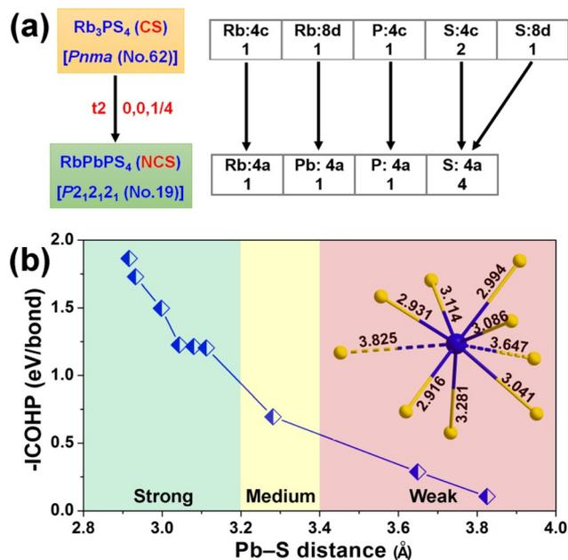
**Fig. 3** (a) Group–subgroup relations between CS Rb<sub>3</sub>PS<sub>4</sub> [space group: *Pnma* (no. 62)] and NCS RbPbPS<sub>4</sub> [space group: *P2<sub>1</sub>2<sub>1</sub>2<sub>1</sub>* (no. 19)]; (b) crystal orbital Hamiltonian population (COHP) curves for the Pb–S bond length in RbPbPS<sub>4</sub> (the inset figure is the coordination geometry of Pb atom).
