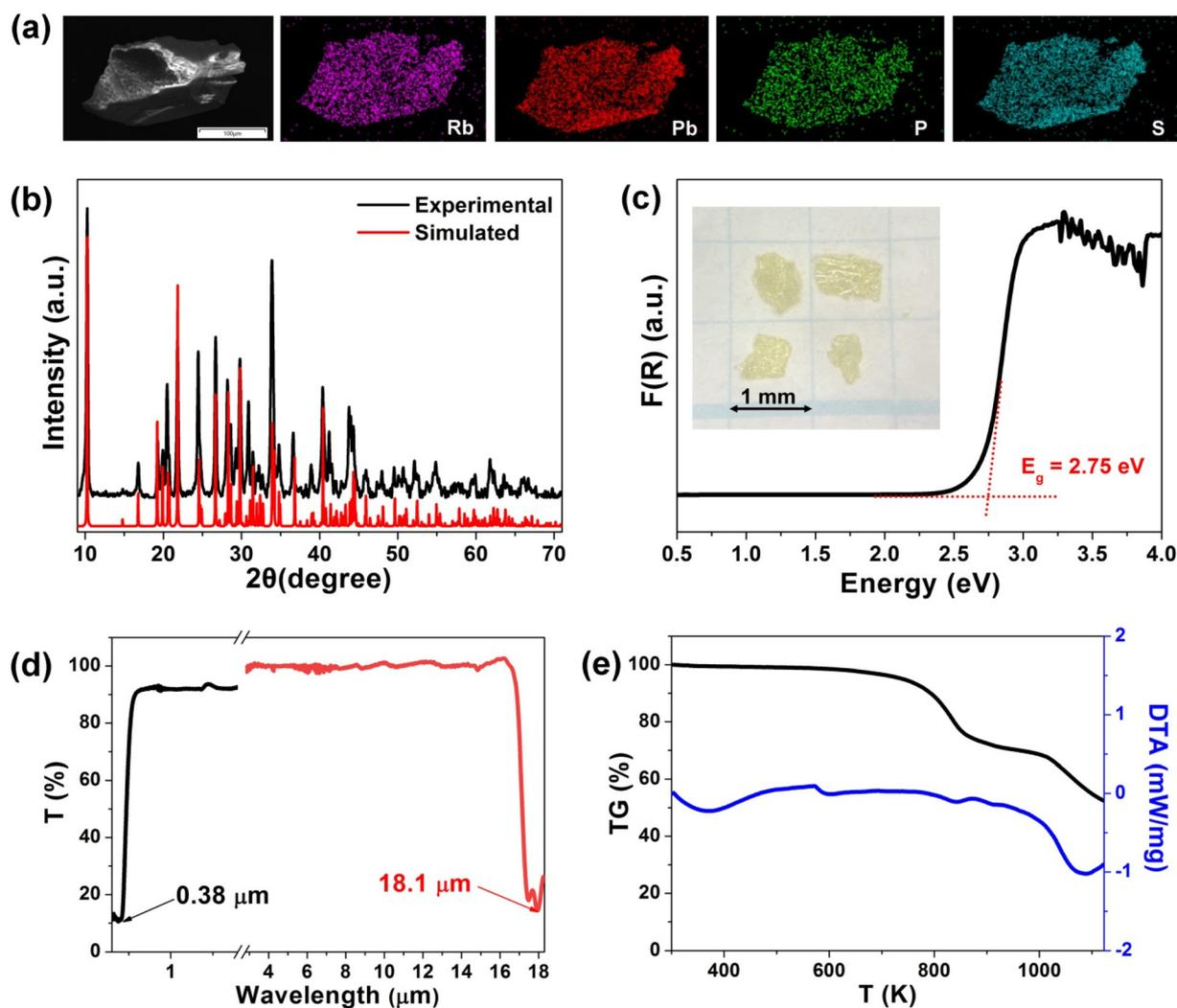
**Fig. 1** Experimental characterization results of  $\text{PbPbPS}_4$ : (a) SEM image and corresponding elemental distribution maps; (b) experimental (black) and simulated (red) powder XRD patterns; (c) UV-vis-NIR spectrum (inset: photograph of the title crystals); (d) optical transmittance spectrum; (e) TG-DTA test curves.
