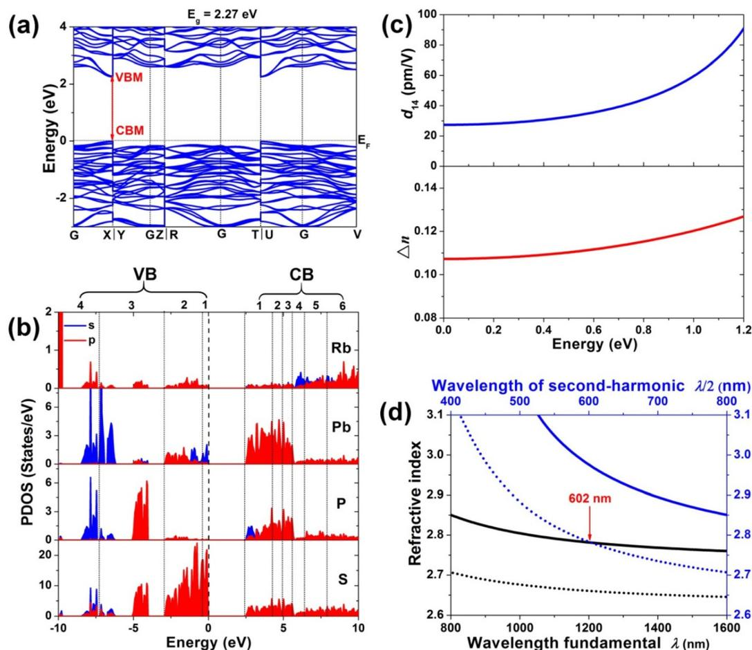
Fig. 5 Theoretical results of electronic structures and optical parameters of  $\text{PbPbPS}_4$ : (a) band structure; (b) partial density of states; (c) calculated nonzero independent SHG coefficient  $d_{14}$  ( $\text{pm V}^{-1}$ ) and calculated birefringence ( $\Delta n$ ); (d) calculated refractive index dispersion curves with the shortest type-I PM cut-off wavelength.
