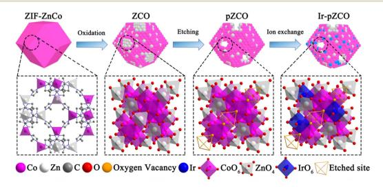
Scheme 1 Schematic of the preparation process for base-etched Ir-pZCO with dispersed Ir species.
