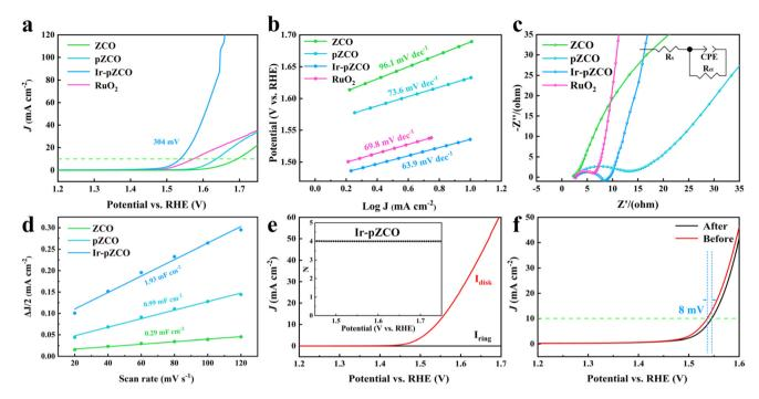
Fig. 4 (a) LSV curves, (b) Tafel plots, (c) EIS analysis, and (d)  $C_{\text{dl}}$  values of all samples. (e) RRDE voltammogram and the calculated N for Ir-pZCO. (f) LSV curves of Ir-pZCO before and after a 10-hour OER.
