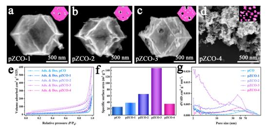
Fig. 1 (a-d) SEM images of the pZCO series. (e-g) N<sub>2</sub> sorption isotherms, BET specific surface area analysis and the corresponding PSD curves of the pCO and pZCO series.
