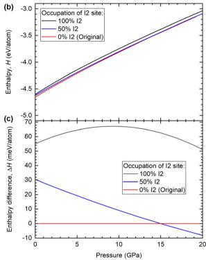
Fig. 6 Enthalpy of competing Ba(IO<sub>3</sub>)<sub>2</sub>·H<sub>2</sub>O configurations according to density functional theory calculations. (a) Calculated enthalpy for the Ba (IO<sub>3</sub>)<sub>2</sub>·H<sub>2</sub>O structure at 12.2 GPa with 0, 12.5, 25, 37.5, 50, 62.5, 75, 87.5 and  $100\% IO_3$  inversion. (b) The enthalpy and (c) enthalpy of the 50 and 100% configurations relative to the 0% configuration.
