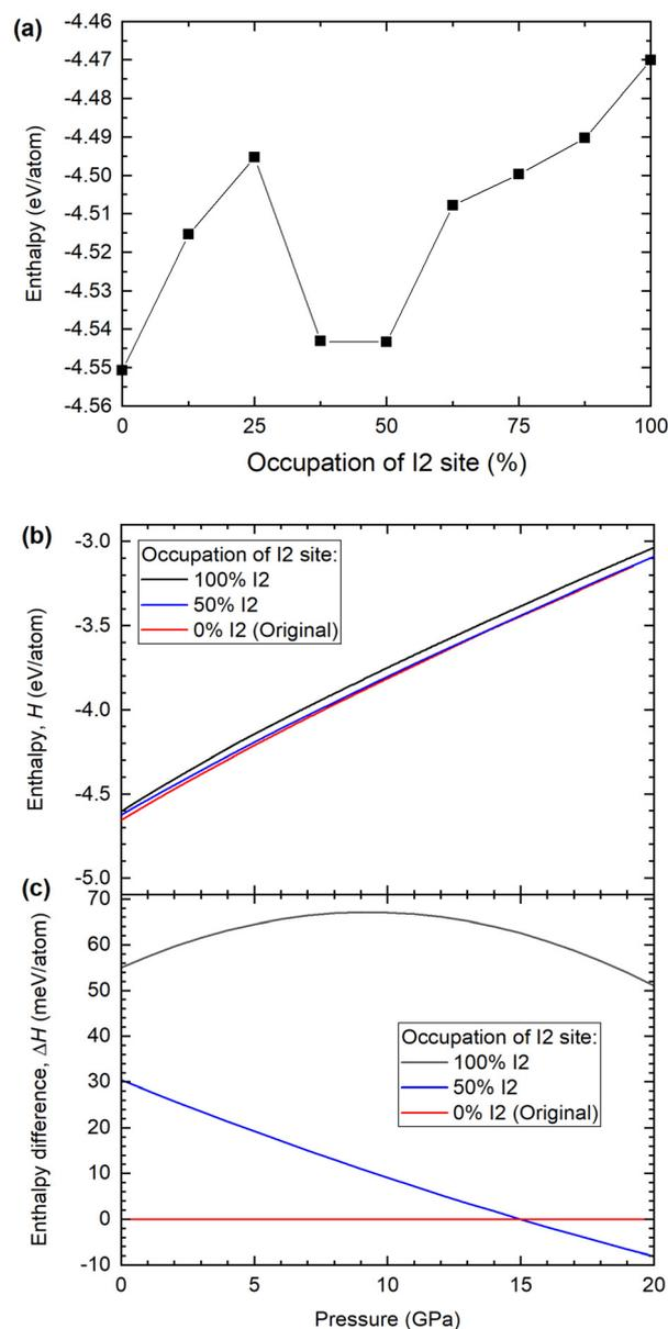
**Fig. 6** Enthalpy of competing  $\text{Ba}(\text{IO}_3)_2 \cdot \text{H}_2\text{O}$  configurations according to density functional theory calculations. (a) Calculated enthalpy for the  $\text{Ba}(\text{IO}_3)_2 \cdot \text{H}_2\text{O}$  structure at 12.2 GPa with 0, 12.5, 25, 37.5, 50, 62.5, 75, 87.5 and 100%  $\text{IO}_3$  inversion. (b) The enthalpy and (c) enthalpy of the 50 and 100% configurations relative to the 0% configuration.
