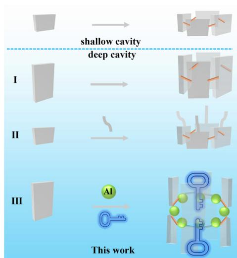
**Scheme 1** Diagram showing the designable assembly of macrocycles. There are three strategies to obtain deep-cavity macrocycles: (I) self-assembly cyclization achieved using long building blocks; (II) postmodification (that is, extending the cavity depth of an existing macrocycle); and (III) self-assembly cyclization as achieved in this work using long building blocks and inorganic aluminum ions, which can trap linear dyes.
