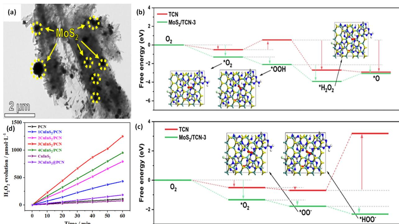
**Fig. 27** (a) SEM images of MoS<sub>2</sub>-/TCN-3. Free energy change graphs for the  $\cdot\text{HO}_2^- 2e^-$  ORR pathway under (b) acidic and (c) alkaline conditions. The figures are adapted with permission from ref. 201. Copyright 2023, Elsevier. (d) Photocatalytic  $\text{H}_2\text{O}_2$  generation by PCN, CuInS<sub>2</sub>, 3CuInS<sub>2</sub>@PCN, and xCuInS<sub>2</sub>/PCN samples. The figures are adapted with permission from ref. 202. Copyright 2023, Elsevier.
