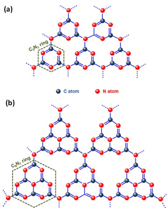
Fig. 5 Structural representation of (a) s-triazine and (b) tri-s-triazine rings within g-C<sub>3</sub>N<sub>4</sub>. The figures are adapted with permission from ref. 88. Copyright 2020, Wiley-VCH.
