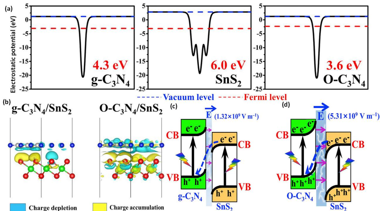
**Fig. 18** (a) Work function values for g-C<sub>3</sub>N<sub>4</sub>, SnS<sub>2</sub>, and O-C<sub>3</sub>N<sub>4</sub> photocatalysts. (b) Charge density variations within the composite photocatalysts. Illustration of the S-scheme charge transfer routes for (c) g-C<sub>3</sub>N<sub>4</sub>/SnS<sub>2</sub> and (d) O-C<sub>3</sub>N<sub>4</sub>/SnS<sub>2</sub> heterojunctions. The figures are adapted with permission from ref. 174. Copyright 2021, Elsevier.
