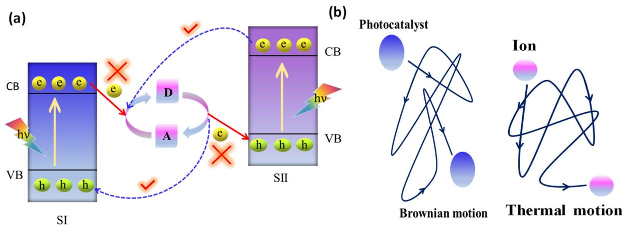
**Fig. 8** (a) Suggested (solid lines) and favored (dotted lines) charge transfer pathways in conventional liquid-phase Z-scheme heterojunctions. (b) Diagrammatic depiction of the Brownian movement of photocatalyst particles and thermal movement of redox couple ions in a solution.
