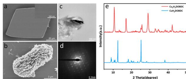
**Fig. 2** (a) SEM images of Cu<sub>2</sub>H<sub>2</sub>DOBDC. (b) SEM images of Cu<sub>2</sub>H<sub>2</sub>DOBDC. (c) TEM images of Cu<sub>2</sub>H<sub>2</sub>DOBDC. (d) SAED pattern of the selected area in (c). (e) XRD patterns of Cu<sub>2</sub>H<sub>2</sub>DOBDC and Cu<sub>2</sub>H<sub>2</sub>DOBDC.
