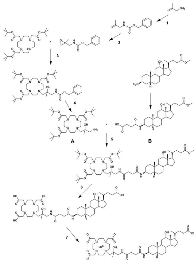
**Scheme 1** Synthetic procedure of Gd-HIBDO3A-DCA and Eu-HIBDO3A-DCA. 1. Benzyl chloroformate 95%, pH 9; 2. MCPBA, RT, 1 day; 3. DIPEA, 60 °C, 6 h; 4. H<sub>2</sub>/Pd, RT; 5. DIPEA, HATU, 24 h, RT; 6. (i) TFA, 24 h, RT, (ii) NaOH 2N (pH 12), 24 h RT, 3 h 50 °C; 7. GdCl<sub>3</sub> or EuCl<sub>3</sub>.
