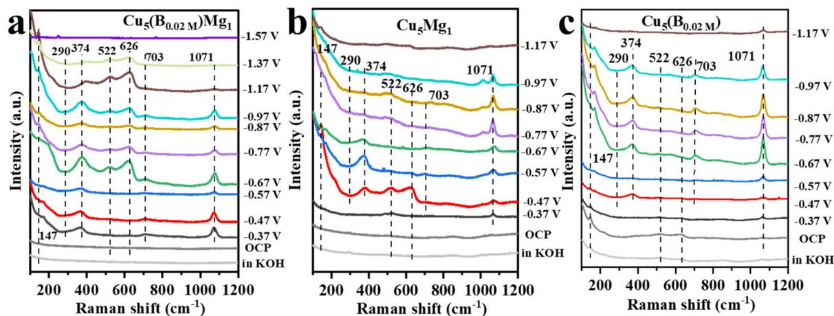
**Fig. 6** The *in situ* Raman spectra of (a)  $\text{Cu}_5(\text{B}_{0.02}\text{M})\text{Mg}_1$ , (b)  $\text{Cu}_5\text{Mg}_1$  and (c)  $\text{Cu}(\text{B}_{0.02}\text{M})$  catalysts at various potentials in 1.0 M KOH electrolyte during  $\text{CO}_2\text{RR}$  catalysis.
