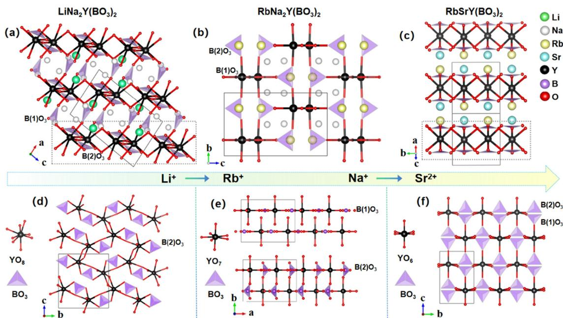
Fig. 1 Structures of (a)  $\text{LiNa}_2\text{Y}(\text{BO}_3)_2$ , (b)  $\text{RbNa}_2\text{Y}(\text{BO}_3)_2$  and (c)  $\text{RbSrY}(\text{BO}_3)_2$ . Connected modes of Y–O and B–O groups in (d)  $\text{LiNa}_2\text{Y}(\text{BO}_3)_2$ , (e)  $\text{RbNa}_2\text{Y}(\text{BO}_3)_2$  and (f)  $\text{RbSrY}(\text{BO}_3)_2$ .
