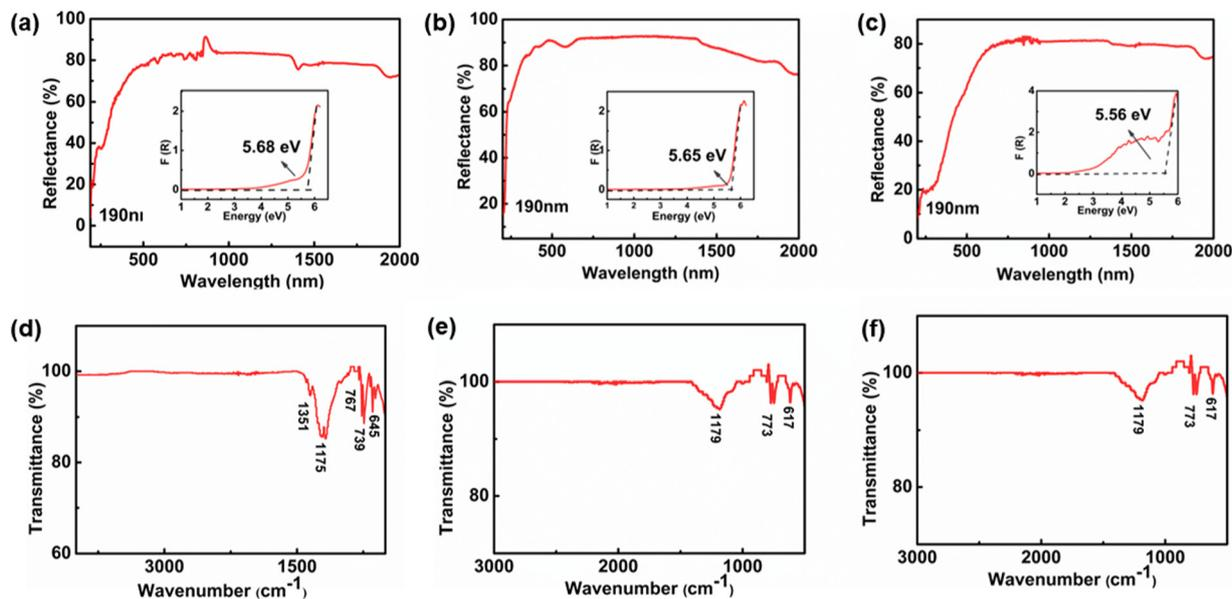
Fig. 2 UV-vis-NIR diffuse reflectance spectra of (a)  $\text{LiNa}_2\text{Y}(\text{BO}_3)_2$ , (b)  $\text{RbNa}_2\text{Y}(\text{BO}_3)_2$ , and (c)  $\text{RbSrY}(\text{BO}_3)_2$ . IR spectra of (d)  $\text{LiNa}_2\text{Y}(\text{BO}_3)_2$ , (e)  $\text{RbNa}_2\text{Y}(\text{BO}_3)_2$ , and (f)  $\text{RbSrY}(\text{BO}_3)_2$ .
