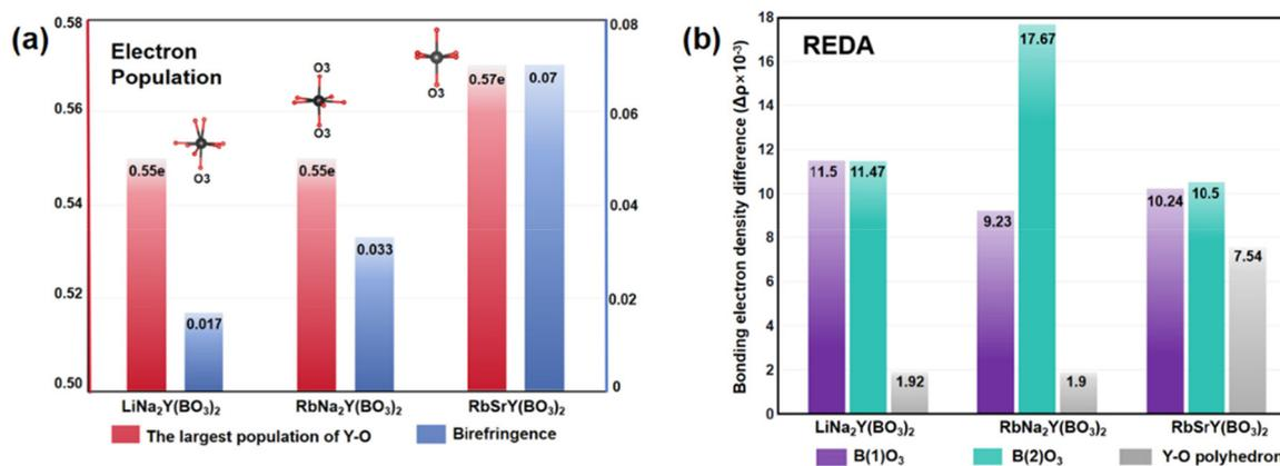
**Fig. 6** (a) Calculated birefringence at 532 nm and the largest population of Y–O bonds. (b) Bonding electron density difference ( $\Delta\rho$ ) of LiNa<sub>2</sub>Y(BO<sub>3</sub>)<sub>2</sub>, RbNa<sub>2</sub>Y(BO<sub>3</sub>)<sub>2</sub>, and RbSrY(BO<sub>3</sub>)<sub>2</sub>.
