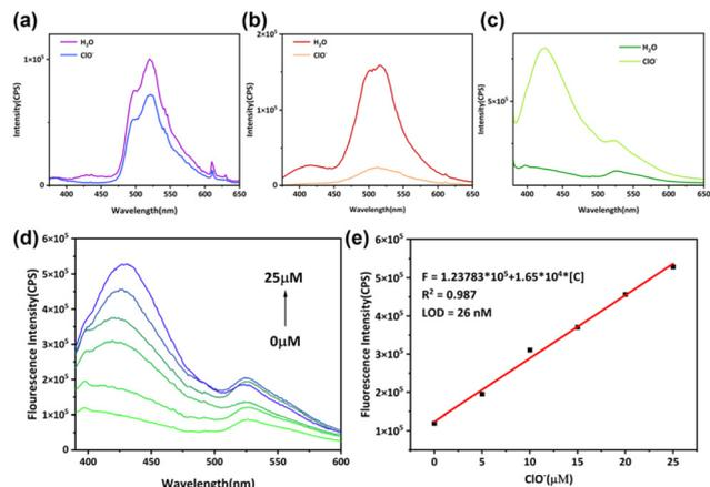
**Fig. 5** PL spectra of PTZ-dbo (a), H<sub>2</sub>PTZ-dba (b) and Cd-PTZ-db (c) in water before and after adding hypochlorite. (d) ClO<sup>-</sup> dose-dependent luminescent spectra of complex Cd-PTZ-db suspensions under optimal sensing conditions and (e) the calibration curve for the detection of ClO<sup>-</sup>.
