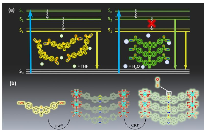
**Scheme 1** (a) Different energy diagrams and relaxation paths of excited state **PTZ-dbo** in tetrahydrofuran (THF) and water. (b) Preparation of **Cd-PTZ-db** and the mechanism of the turn-on luminescence of **Cd-PTZ-db** in response to  $ClO^-$  (red spheres represent O atoms, and cyan spheres represent Cd atoms).
