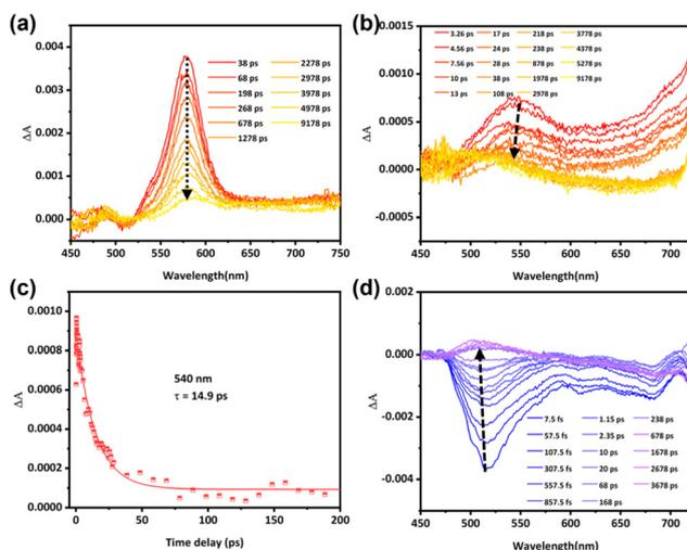
**Fig. 4** (a) fs-TA spectra of  $H_2$ PTZ-dba in THF; (b) fs-TA spectra of  $H_2$ PTZ-dba in the film state; (c) kinetic traces of the  $H_2$ PTZ-dba film at 540 nm. The excitation wavelength is 355 nm. (d) fs-TA spectra of **PTZ-dbo** in the film state. Films were prepared by natural evaporation of their THF solution of 1 mM on a quartz substrate.
