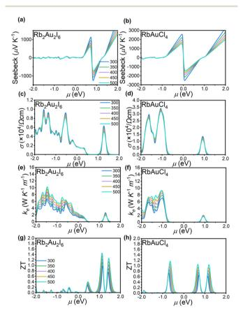
Fig. 5 (a and b) Dependence of chemical potential for Rb<sub>2</sub>Au<sub>2</sub>I<sub>6</sub> and RbAuCl<sub>4</sub> on the Seebeck coefficient; (c and d) electrical conductivity ( $\sigma$ ); (e and f) temperature electronic thermal conductivity ( $\kappa_e$ ); and (g and h) thermoelectric figure of merit (ZT) at different temperatures.
