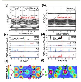
Fig. 3 Electronic band structures and PDOS of compounds (a and c) Rb<sub>2</sub>Au<sub>2</sub>I<sub>6</sub> and (b and d) RbAuCl<sub>4</sub>. Electron localization function contour plots of (e) Rb<sub>2</sub>Au<sub>2</sub>I<sub>6</sub> and (f) RbAuCl<sub>4</sub> (displayed on the (1, 1, -1) lattice plane).
