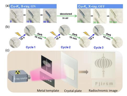
Fig. 3 Radiochromic behavior for RCS-2: (a) time-dependent images for crystalline samples of RCS-2 upon irradiation of Cu-K<sub>rr</sub> X-rays. (b) Colored-decolored cycles of a single-crystal sample upon irradiation of Cu-K<sub>u</sub>. (c) Radiochromism imaging. (The photographs of (a) and (b) were both captured in their original context.)
