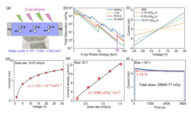
Fig. 2 Single-crystal X-ray detection performance of RCS-2: (a) schematic illustration of the X-ray detector and actual electrode diagram. (b) Calculated mass attenuation coefficients. (c) I-V curves under X-ray off and on with different exposed dose rates. (d) Voltage-dependent photocurrent curves fitted by the Hecht equation. (e) Photocurrent density versus dose rate measured at a bias voltage of 30 V. (f) Device stability in air under continuous X-ray irradiation.
