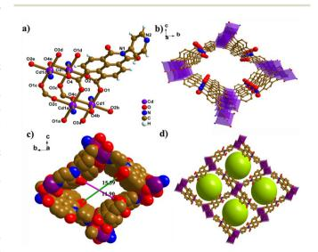
Fig. 1 Crystal structure of CdPNMI. (a) Representation of the Cd coordination environment; (b) 3D net with abundant nitrogen and oxygen sites along the inner channel walls; (c) space-filling model of a 1D channel viewed along the *a*-axis; (d) view of 1D channels along the *a* axis filled with green balls.
