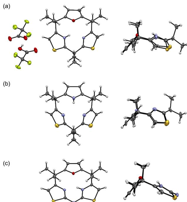
**Fig. 2** Single crystal X-ray structures (left, top view; right, side view) of (a) **5·TFA**, (b) **2**, and (c) **10** drawn at the 50% probability level of the thermal ellipsoids (H, white; C, gray; N, blue; O, red; S, yellow; and F, yellow green).
