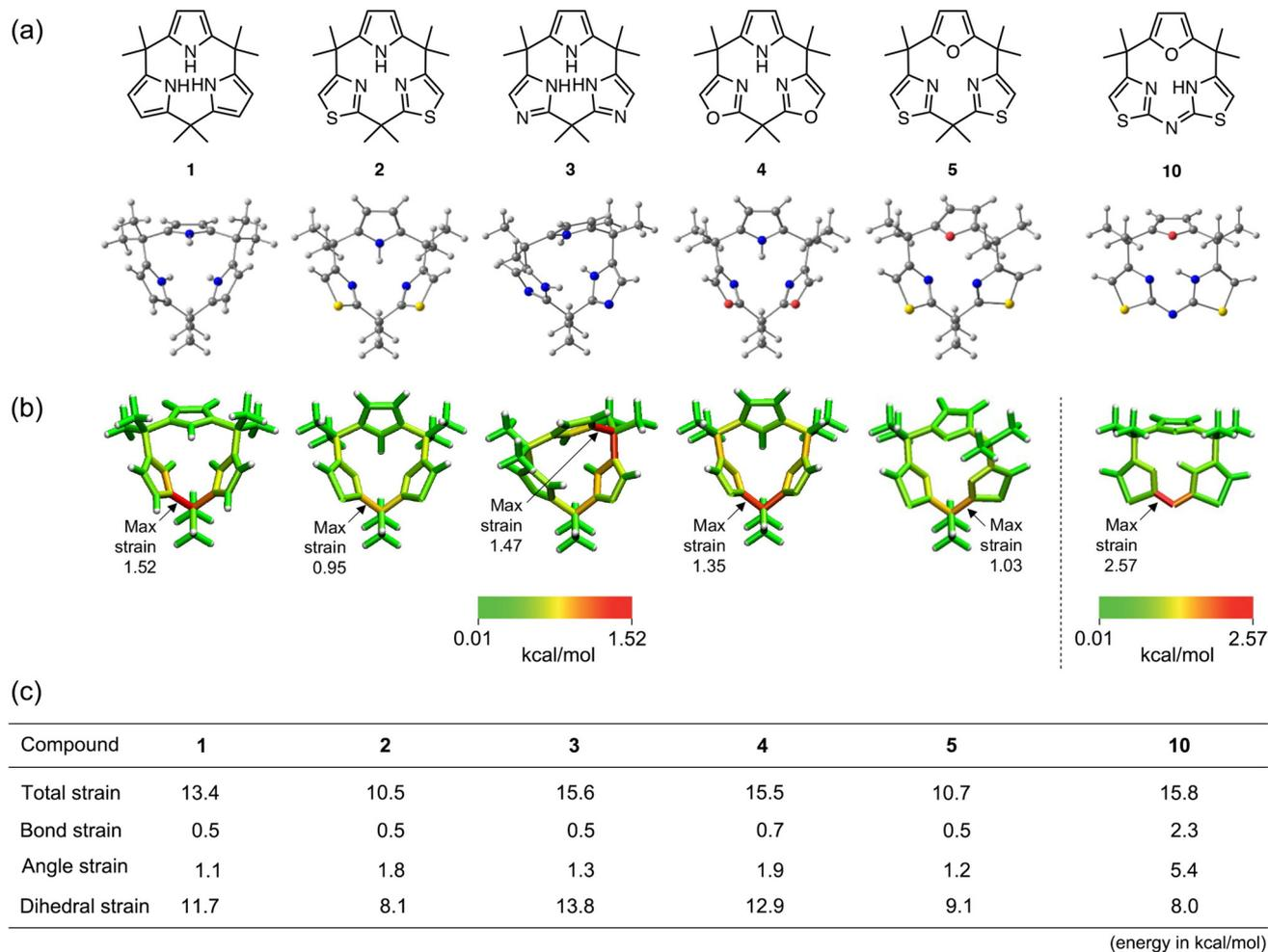
**Fig. 1** (a) Optimized structures of the lowest energy conformations of calix[3]pyrrole (**1**) and its analogues **2–5**, and **10**. (b) Visualization of the total ring strain of **1–5** and **10** using the StrainViz analysis. (c) Calculated total, bond, angle, and dihedral strain energies of **1–5** and **10** (in kcal mol<sup>-1</sup>).
