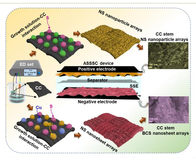
Fig. 1 A schematic representation displaying the simple synthesis of BCS-x and NS on a flexible CC current collector and assembly of the ASSSC device.
